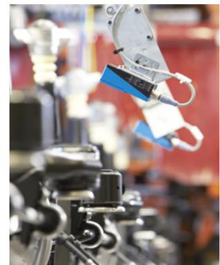
Part inspection and dimensioning in automotive assembly
