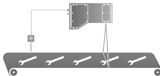
The IVC-3D scans height profiles into a 3D image as the objects move by on the conveyor.
