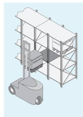
◀ When the DMP is used, a reflector is fixed on each bin and reflects the light emitted by the DMP. The DMP evaluates this reflected light. The reflectors are fixed reference points, which make reliable positioning possible even when the ambient conditions change.
