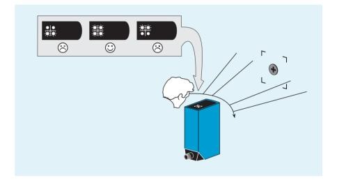
No special settings or programming of the DMP is required. The DMP Position Finder must only be aimed at the reflector, and then it is ready to operate. When operation of the DMP is started, all four control lamps light for a brief time (→ function test).
