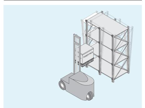
▲ In high-bay storage bins, there can be tolerance-dependent storage measurements due to uneven warehouse floors in addition to material-dependent tolerances in the construction. These tolerances do not influence the accuracy of the DMP.
