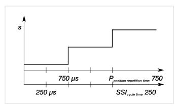
NOTE: The SSI cycle (cyclic access to the LinCoder® by controller/regulator) of 250 µs is assumed here.
