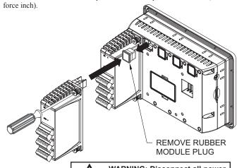
WARNING: Disconnect all power to the unit before installing or removing modules.
