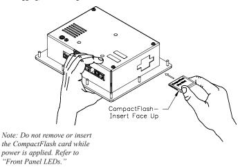
Information stored on a CompactFlash card by a G306 can be read by a card reader attached to a PC. This information is stored in IBM (Windows®) PC compatible FAT16 file format.
