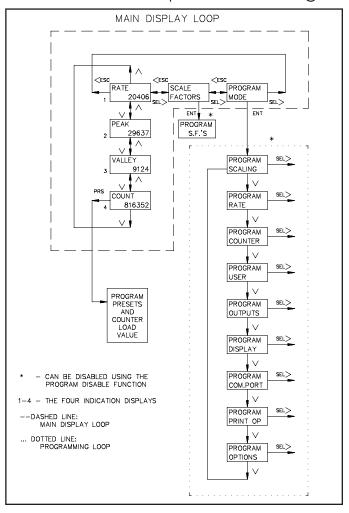
significant digits on the 6-digit Rate display. The desired time units that the rate is to be displayed, can also be programmed as per Second (x1), per Minute (x60), or per Hour (x3600).
