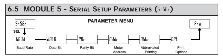
The Serial Setup Parameters are only active when one of the optional serial communication/programming cards is installed in the meter.
