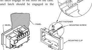
farthest forward slot possible. To achieve a proper seal, tighten the latch screws evenly until the unit is snug in the panel (Torque to approx. 28 to 36 in-oz [0.202 to 0.26 N-m]). Do not over-tighten the screws.
