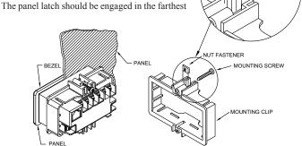
forward slot possible. To achieve a proper seal, tighten the latch screws evenly until the unit is snug in the panel (Torque to approx. 28 to 36 in-oz [0.202 to 0.26 N-m]). Do not over-tighten the screws.
