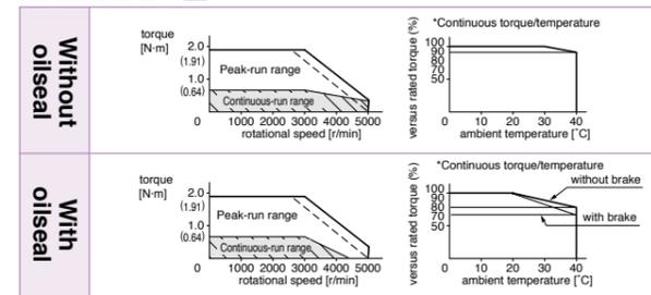
\*When you lower the torque limit setup (Pr5E and 5F), running range at high speed might be lowered as well.
