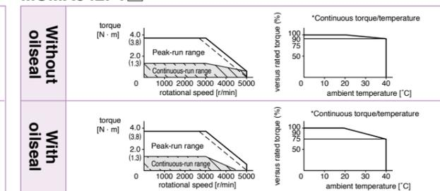
\*When you lower the torque limit setup (Pr5E and 5F), running range at high speed might be lowered as well.
