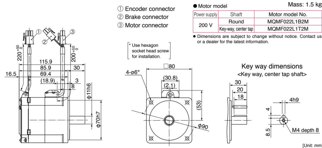
Leadwire type (IP65) • with brake • with oil seal • Round shaft/ Key way, center tap shaft
