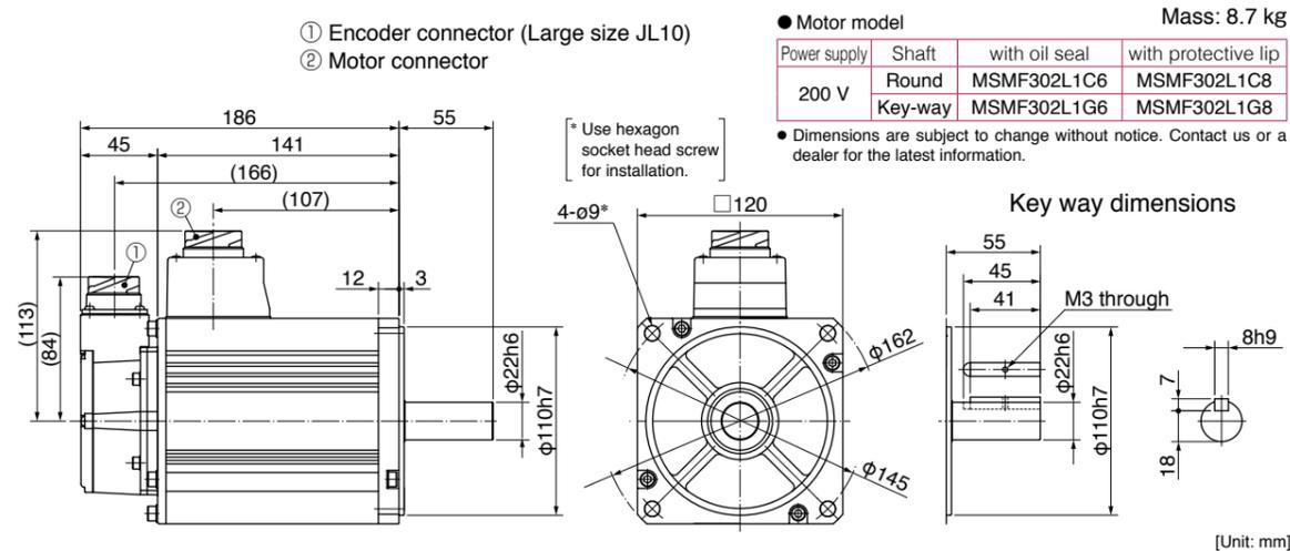
Large size connector (JL10) type · with brake · with oil seal/ with protective lip · Key way shaft/ Round shaft
