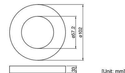
Fig.2: RJ8095 (Recommended components) 1 pieces
