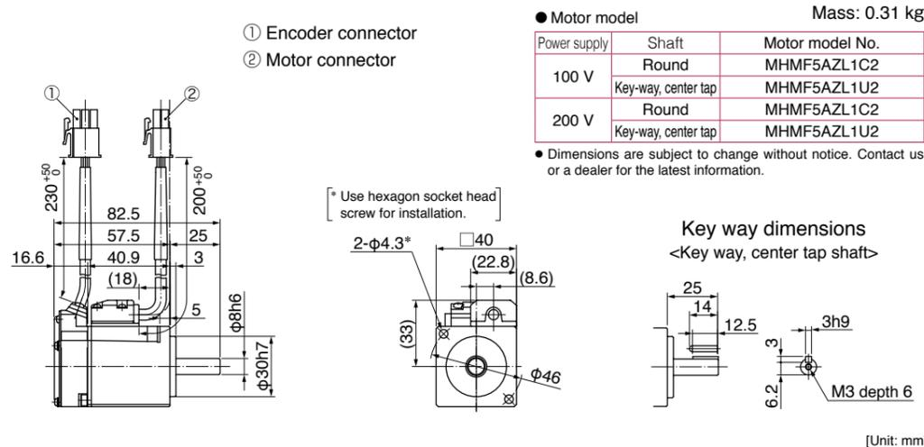
Leadwire type (IP65) • without brake • with protective lip/ with oil seal • Round shaft/ Key way, center tap shaft
