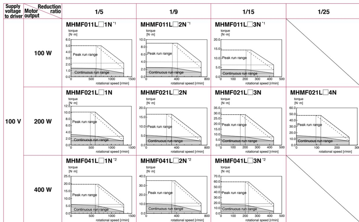
Dotted line represents the torque at 10% less supply voltage to driver.
