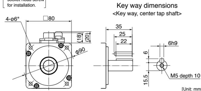
Connector type (IP67) • with brake • without/with oil seal • Round shaft/ Key way, center tap shaft
