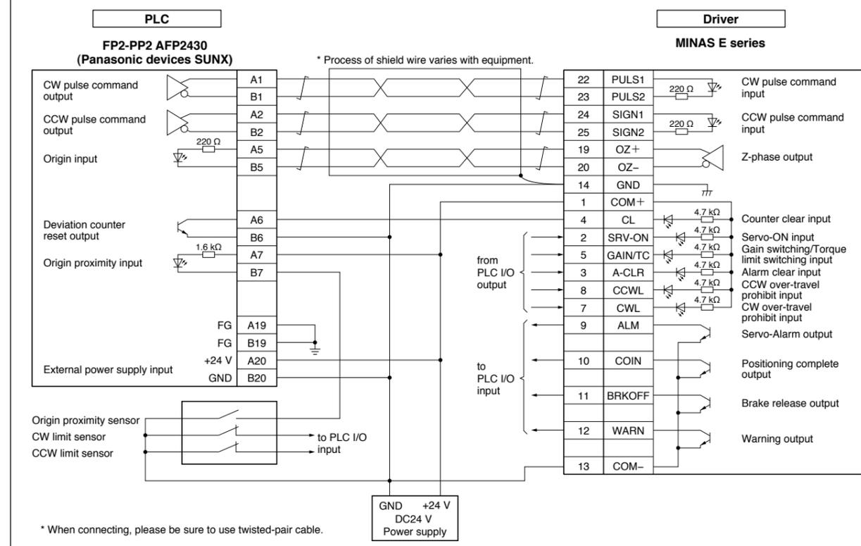
**AFP0HPG01L(1-axes)/AFP0HPG02L(2-axes) Connection with the Panasonic devices SUNX.**
