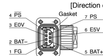
• Pin disposition of connector for motor cable
