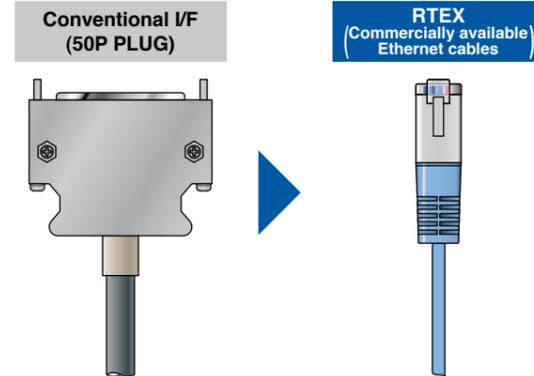
Maximum length of the node-to-node cable is 100 m.
