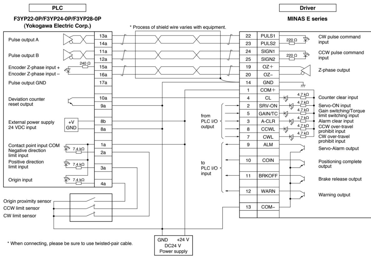
**CJ1W-NC113 Connection with the Omron Corp.**
