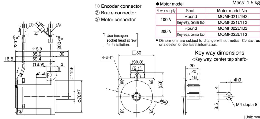
Leadwire type (IP65) • with brake • with oil seal • Round shaft/ Key way, center tap shaft
