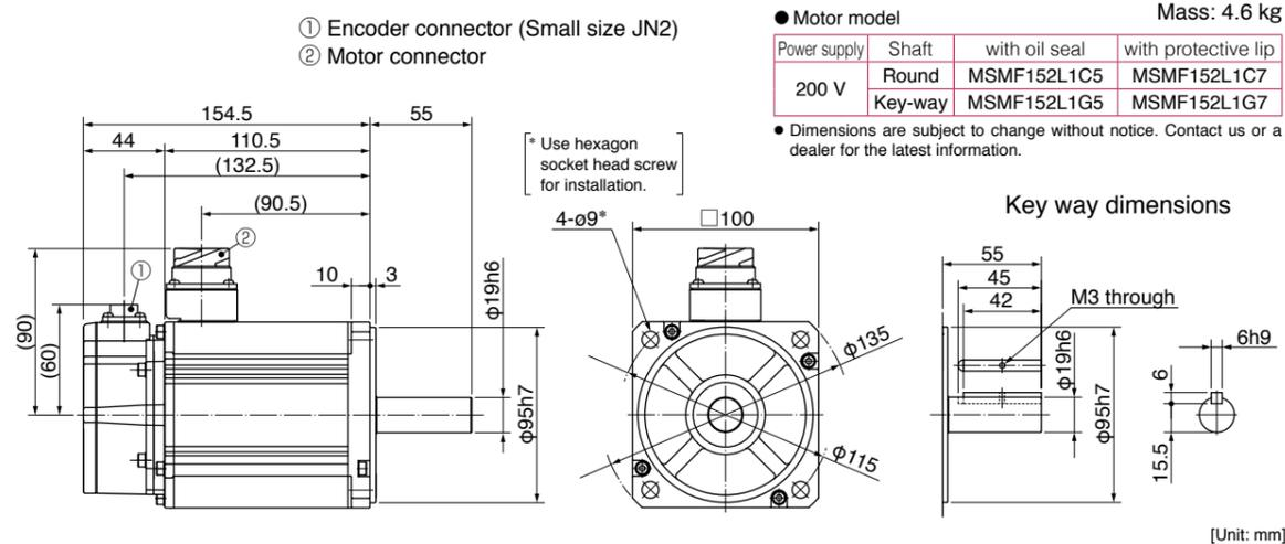
Small size connector (JN2) type · with brake · with oil seal/ with protective lip · Key way shaft/ Round shaft
