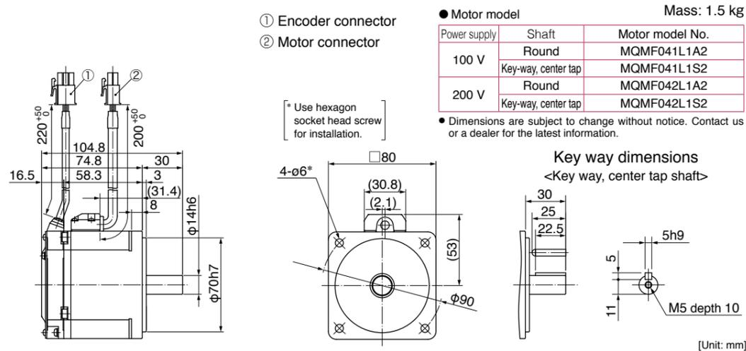
Leadwire type (IP65) • without brake • with oil seal • Round shaft/ Key way, center tap shaft
