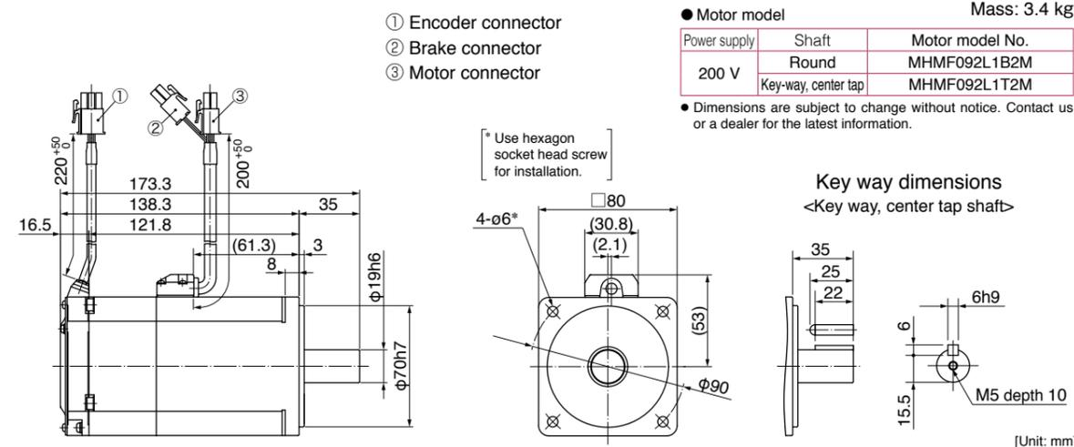
Leadwire type (IP65) • with brake • with oil seal • Round shaft/ Key way, center tap shaft
