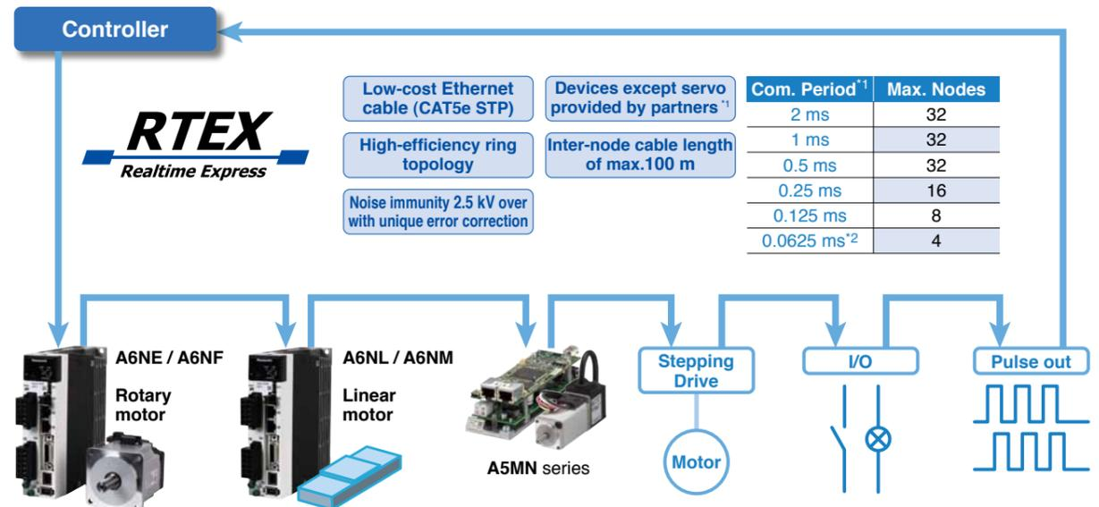
\*1: The communication period and connection of slave devices depend on the controller specification.
