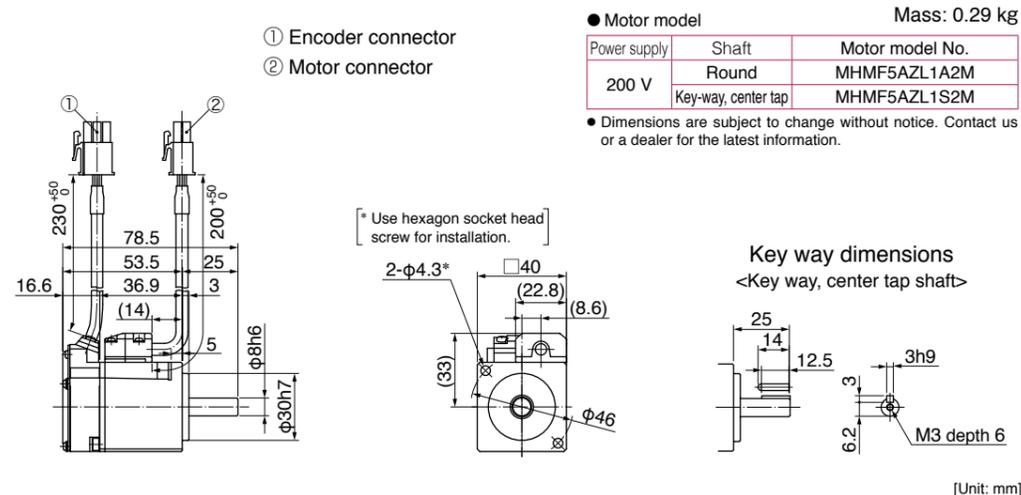
Leadwire type (IP65) • without brake • with oil seal • Round shaft/ Key way, center tap shaft
