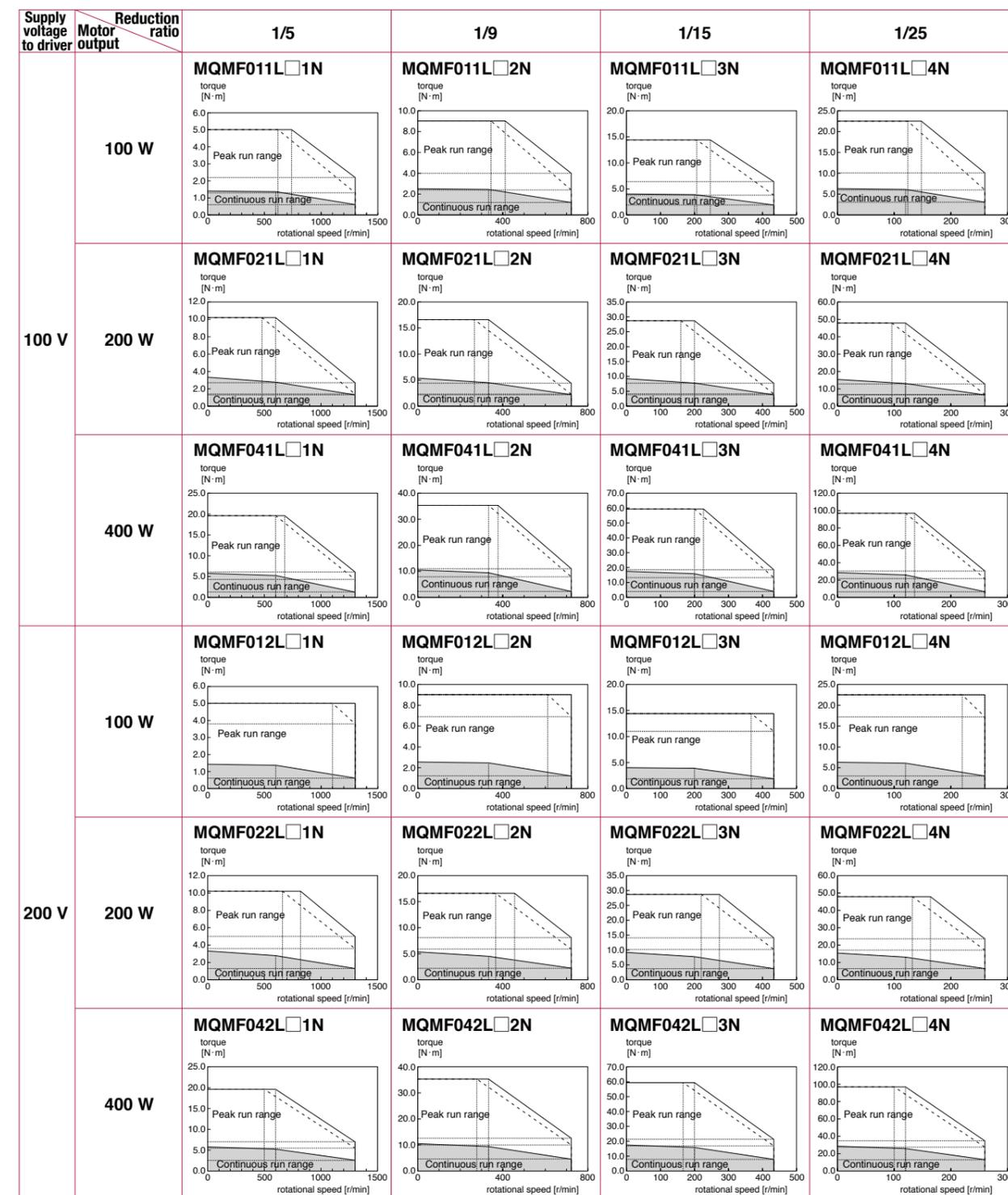
Dotted line represents the torque at 10 % less supply voltage to driver.
