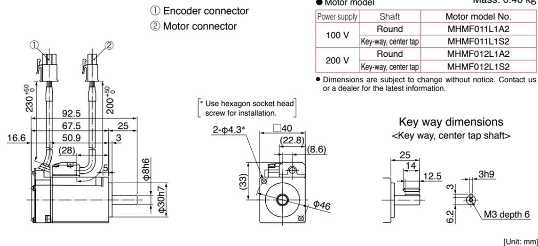
Leadwire type (IP65) • without brake • with oil seal • Round shaft/ Key way, center tap shaft
