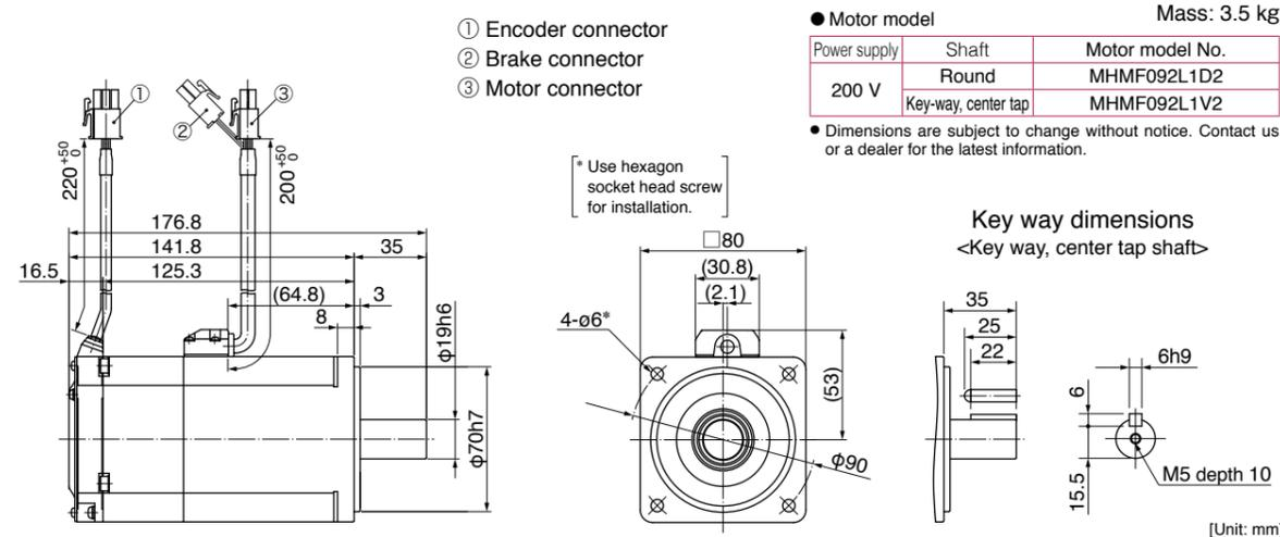
Leadwire type (IP65) • with brake • with protective lip/ with oil seal • Round shaft/ Key way, center tap shaft
