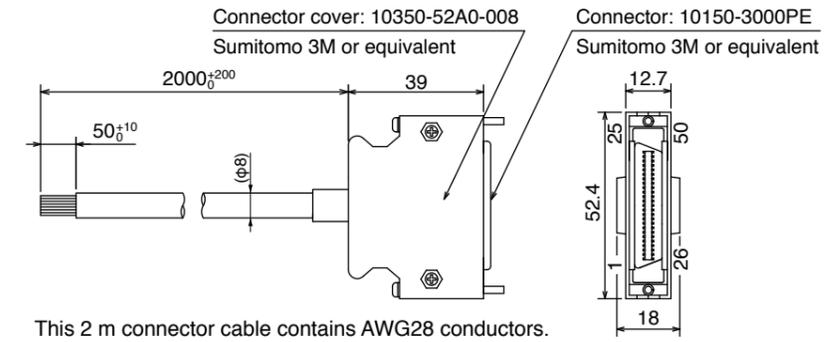
This 2 m connector cable contains AWG28 conductors.
