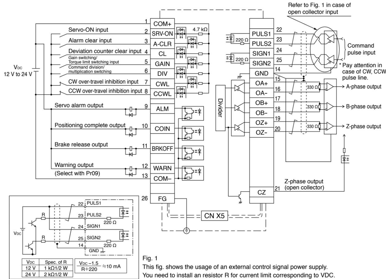
CN X 5 Wiring Example at Internal Velocity Control Mode
