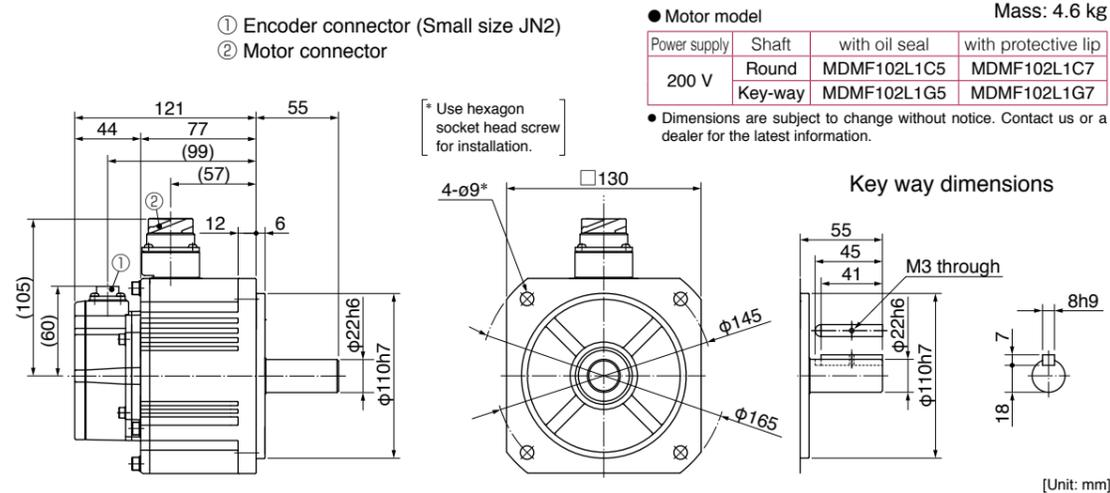
Small size connector (JN2) type · with brake · with oil seal/ with protective lip · Key way shaft/ Round shaft
