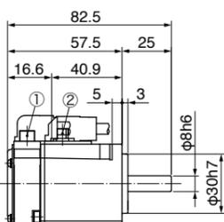
\* Use hexagon socket head screw for installation.
