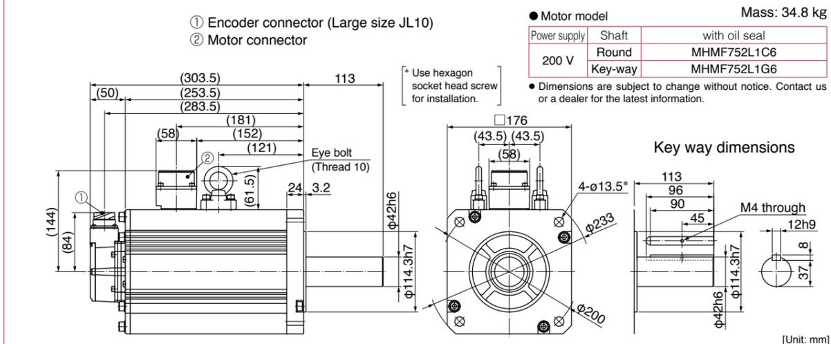
Large size connector (JL10) type • with brake • with oil seal • Key way shaft/ Round shaft
