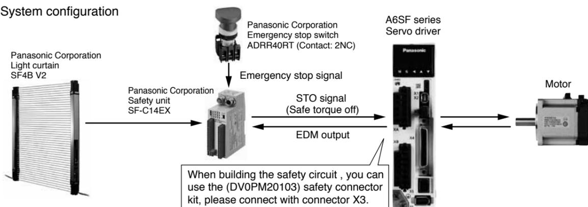
When building the safety circuit, you can use the (DV0PM20103) safety connector kit, please connect with connector X3.
