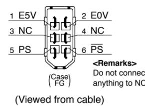
• Pin disposition of connector for encoder cable
