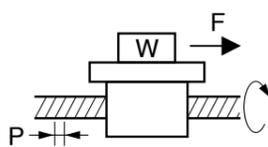
Traveling torque  $T_f = \frac{P}{2\pi\eta} (\mu gW + F)$
