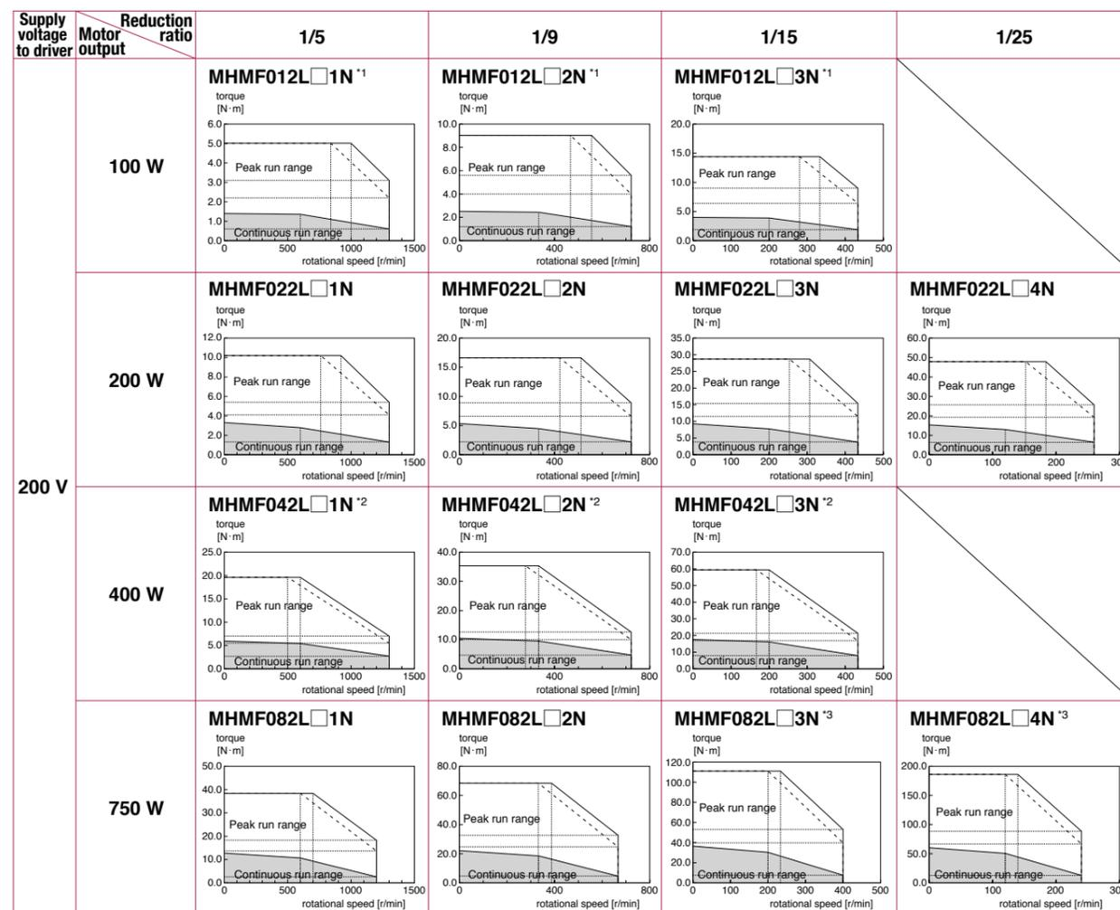
Dotted line represents the torque at 10% less supply voltage to driver.
