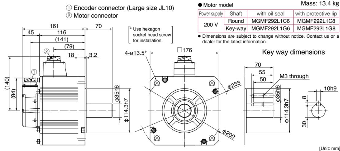
Large size connector (JL10) type · with brake · with oil seal/ with protective lip · Key way shaft/ Round shaft
