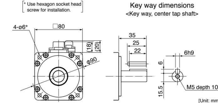
Connector type (IP67) • with brake • without/with oil seal • Round shaft/ Key way, center tap shaft
