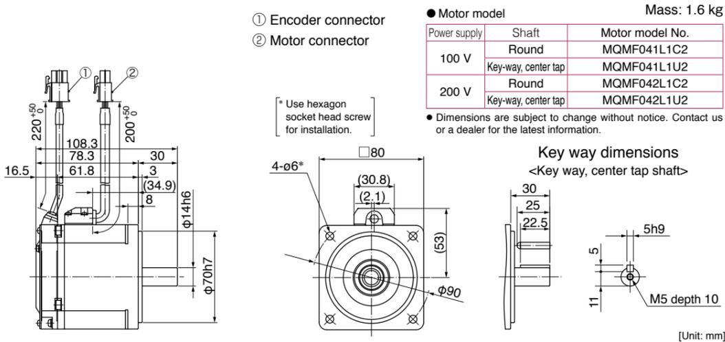
Leadwire type (IP65) • without brake • with protective lip/ with oil seal • Round shaft/ Key way, center tap shaft
