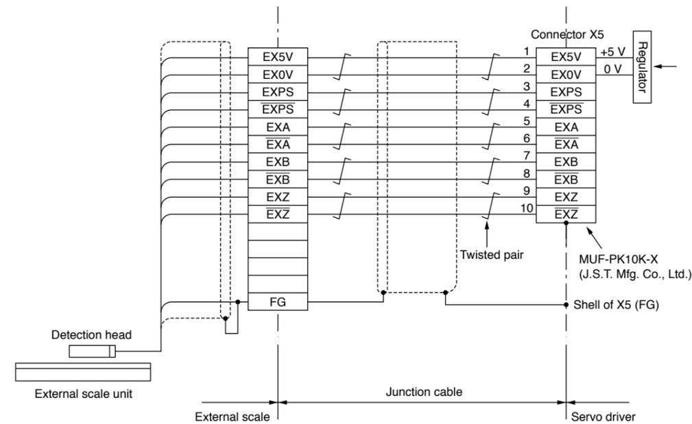
When using a 23-bit absolute encoder as an absolute system\*.
