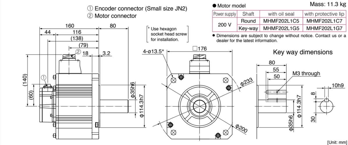
Small size connector (JN2) type · with brake · with oil seal/ with protective lip · Key way shaft/ Round shaft
