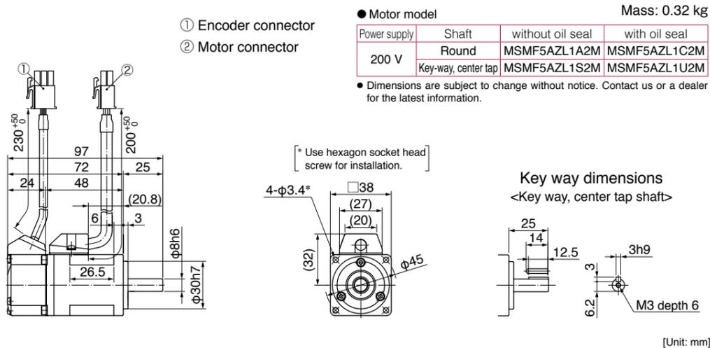
Leadwire type (IP65) • with brake • without/with oil seal • Round shaft/ Key way, center tap shaft
