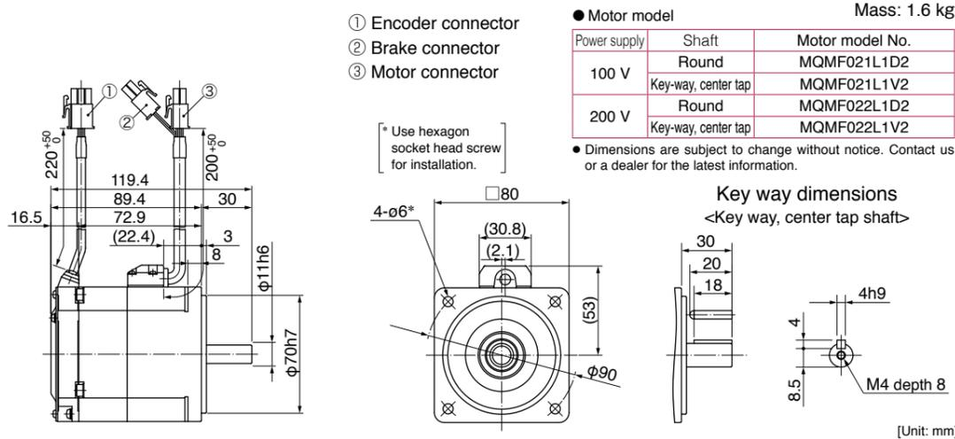
Leadwire type (IP65) • with brake • with protective lip/ with oil seal • Round shaft/ Key way, center tap shaft
