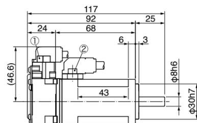
\* Use hexagon socket head screw for installation.
