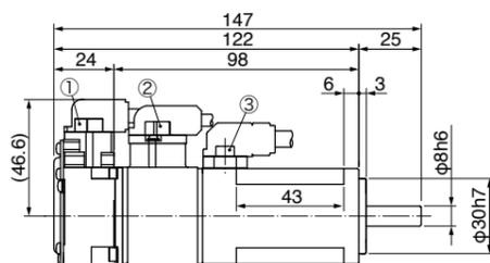
\* Use hexagon socket head screw for installation.
