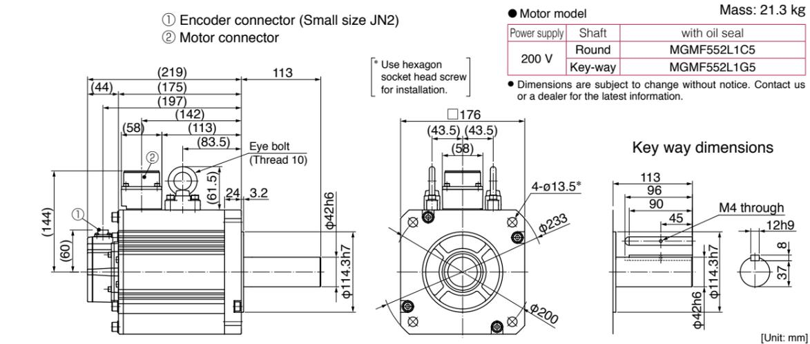
Small size connector (JN2) type · with brake · with oil seal · Key way shaft/ Round shaft
