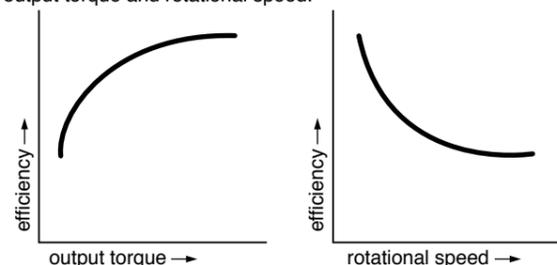
**Specifications of Motor with Gear Reducer**
