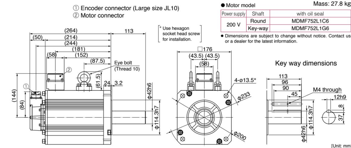
Large size connector (JL10) type · with brake · with oil seal · Key way shaft/ Round shaft
