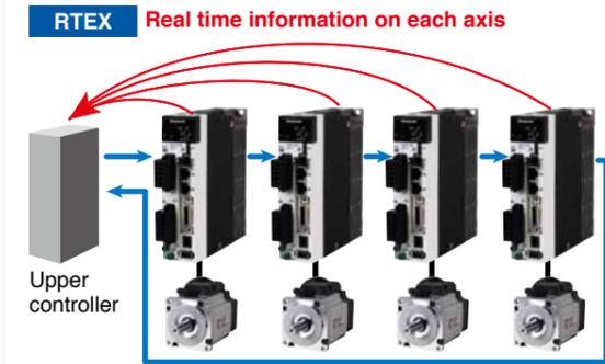
Up to 32 axes can be controlled.
