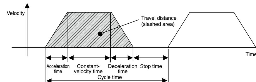
Note) Selection of motor capacity significantly varies depending on the operating pattern. The motor capacity can be reduced if the acceleration/deceleration time and stop time are set as long as possible.
