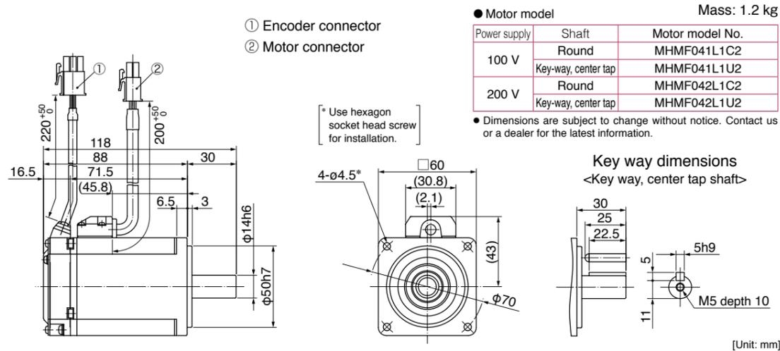
Leadwire type (IP65) • without brake • with protective lip/ with oil seal • Round shaft/ Key way, center tap shaft
