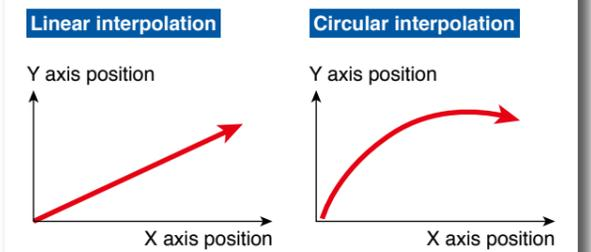
\* Interpolation depends on the specification of upper controllers. This is not the function of individual servo motor.
