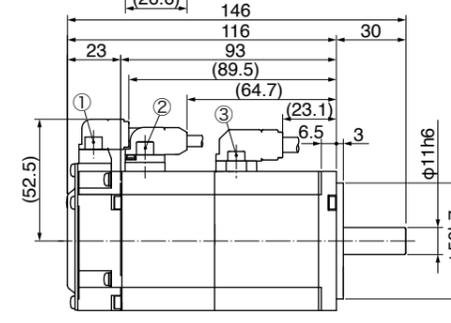
\* Use hexagon socket head screw for installation.
