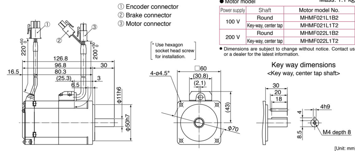
Leadwire type (IP65) • with brake • with oil seal • Round shaft/ Key way, center tap shaft
