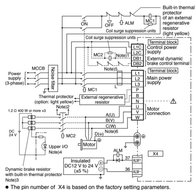
• The pin number of X4 is based on the factory setting parameters.
