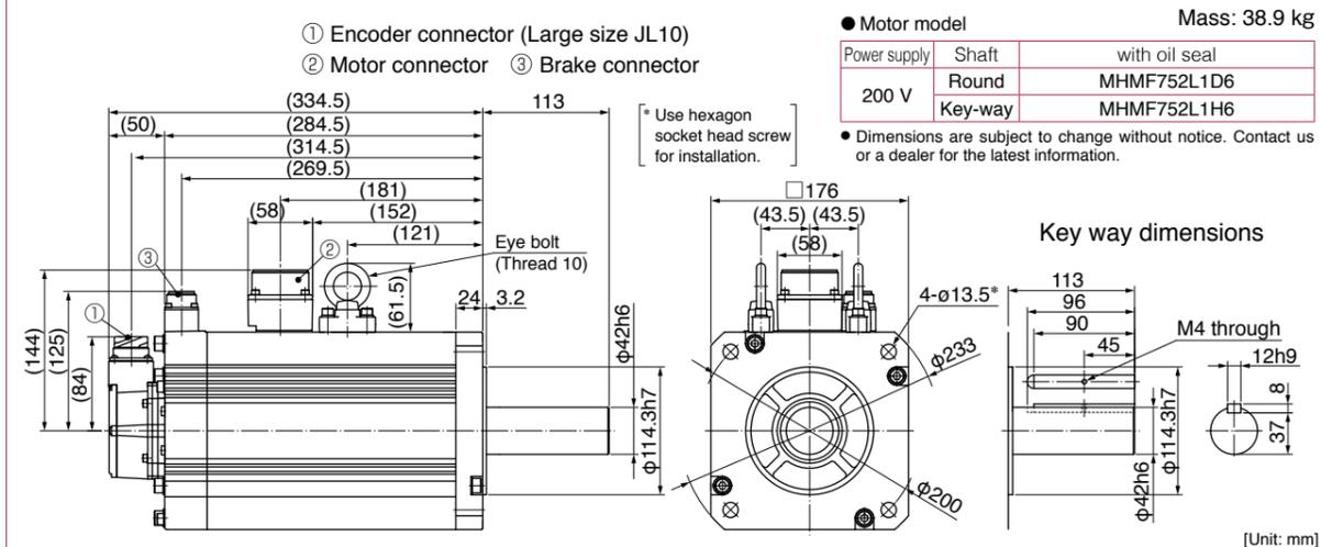
Small size connector (JN2) type • without brake • with oil seal • Key way shaft/ Round shaft
