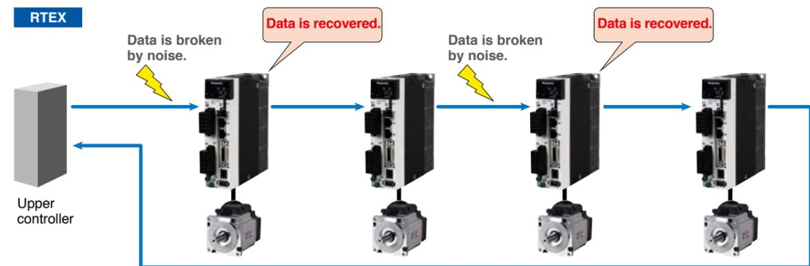
\* The error correction function has a limit. Unrecovered broken data causes a communication error.
