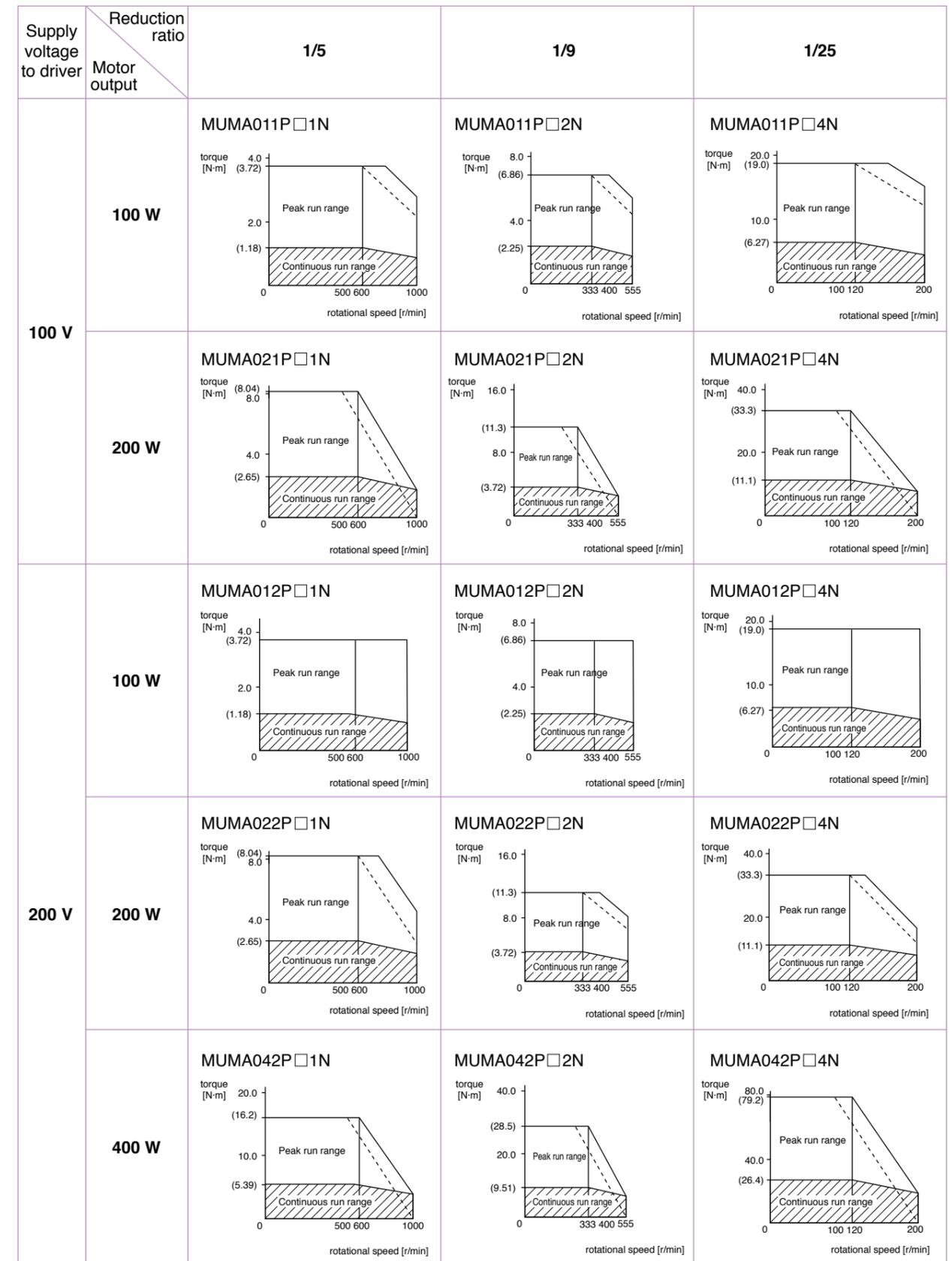
Dotted line represents the torque at 10 % less supply voltage.
