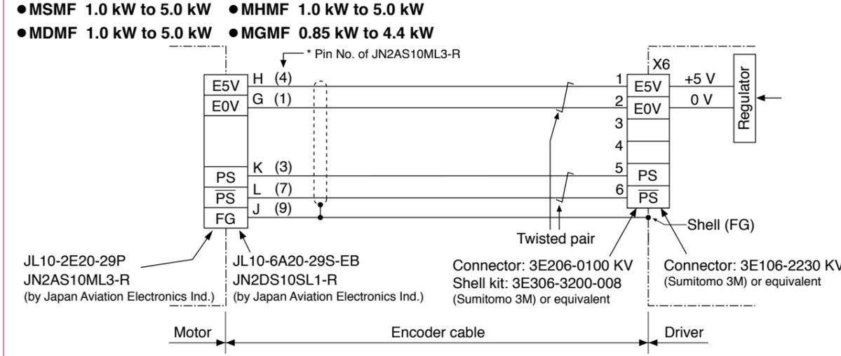
[Connector pin assignment] Refer to P.307, P.308 "Specifications of Motor connector".
