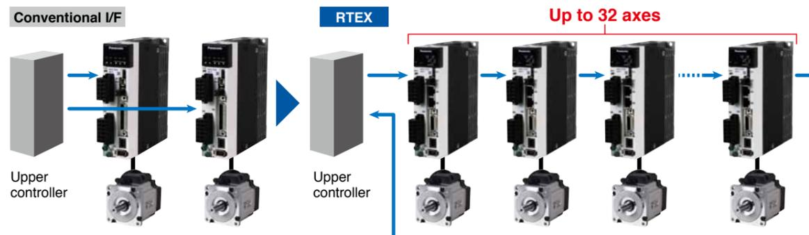
\* If devices other than servo motors are also connected, up to 32 nodes can be connected as entire slaves including the servo motors. Actual number of controllable axes depends on the specification of an upper controller.
