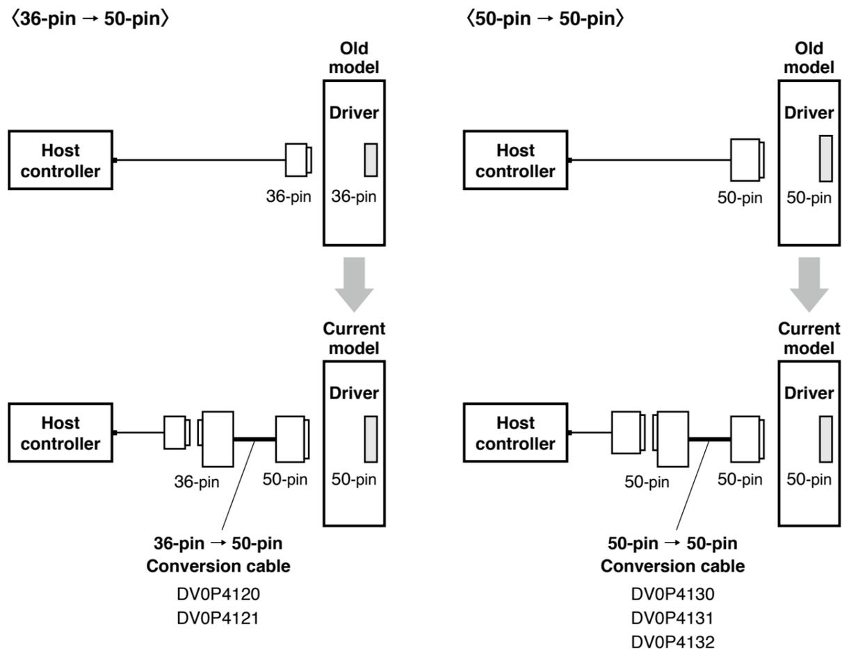
When selecting the cable, refer to the table below because the part number of the cable is specific to the control mode of the old model.
