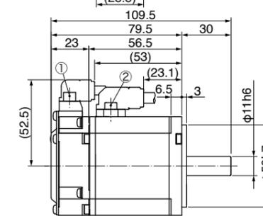
\* Use hexagon socket head screw for installation.
