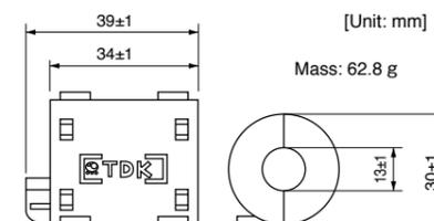
Fig.3: T400-61D (Recommended components) 1 pieces
