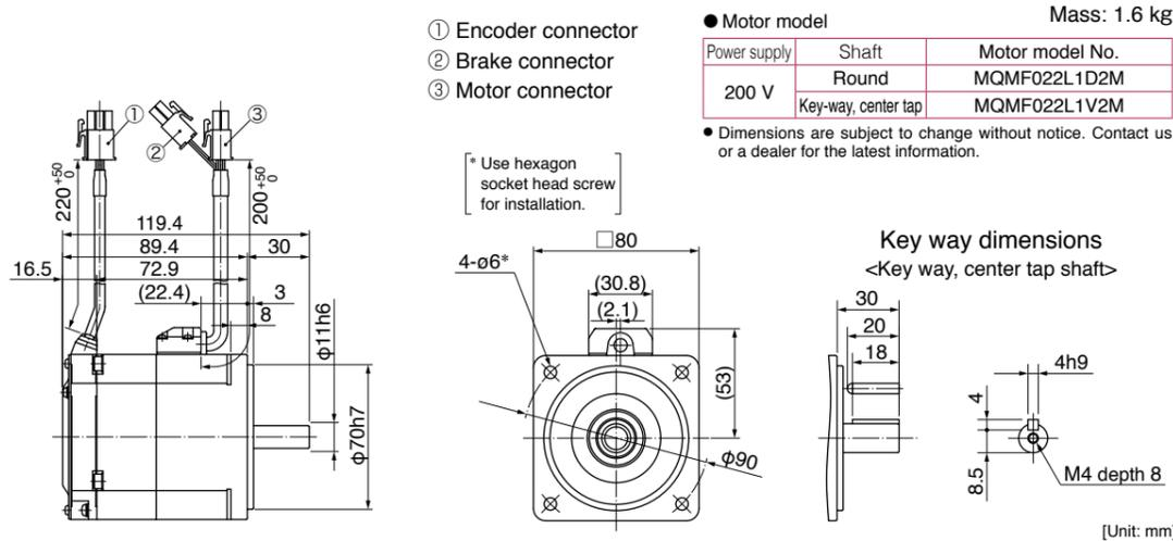
Leadwire type (IP65) • with brake • with protective lip/ with oil seal • Round shaft/ Key way, center tap shaft
