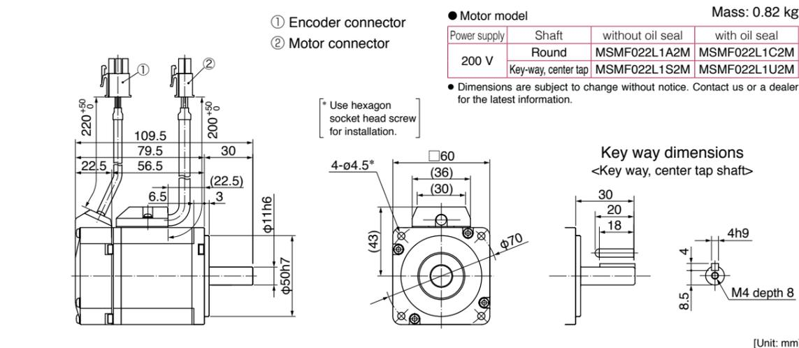
Leadwire type (IP65) • with brake • without/with oil seal • Round shaft/ Key way, center tap shaft
