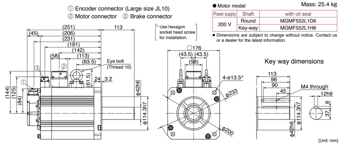
Small size connector (JN2) type · without brake · with oil seal · Key way shaft/ Round shaft
