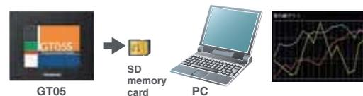
The trigger can be selected from among time, frequency (1sec to 24hrs), and conditions (external trigger). Data can be saved for up to 6,000 entries per type and up to 16 types.\*
