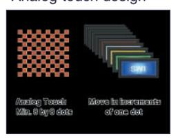
You can freely position switches as small as 8 x 8 dots.
