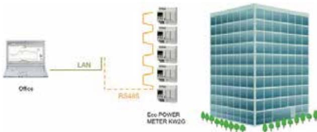
Use the FP7 together with a Eco-POWER METER to monitor the energy consumption of each floor in a building.
