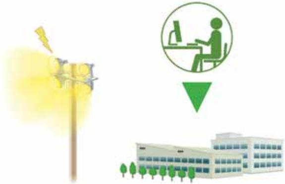
Use the FP7 together with an Eco-POWER METER such as KW2G and a wireless unit to gather data from exterior lighting systems and monitor energy consumption. Data can be logged and visualized remotely on an office PC with the FP Data Analyzer software.
