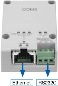
Enables easy Ethernet connections with a compact PLC, which were previously not possible. Also equipped with an RS232C port. Together with the tool port (programming port), a total of 3 communication ports are available, which is remarkable for a compact PLC.
