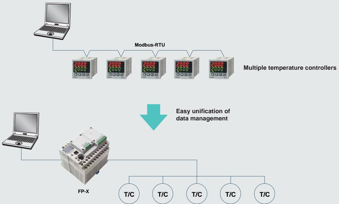
For connecting a thermocouple, please use an FP0 thermocouple unit via an adapter (AFPX-EFP0).
