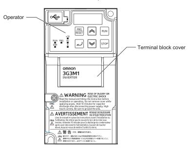
Open the terminal block cover to wire the main circuit terminal block and the control circuit terminal block.
