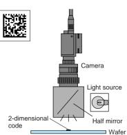
The following descriptions are based on the Data Matrix and QR Code systems, both of which use 2-dimensional codes.
