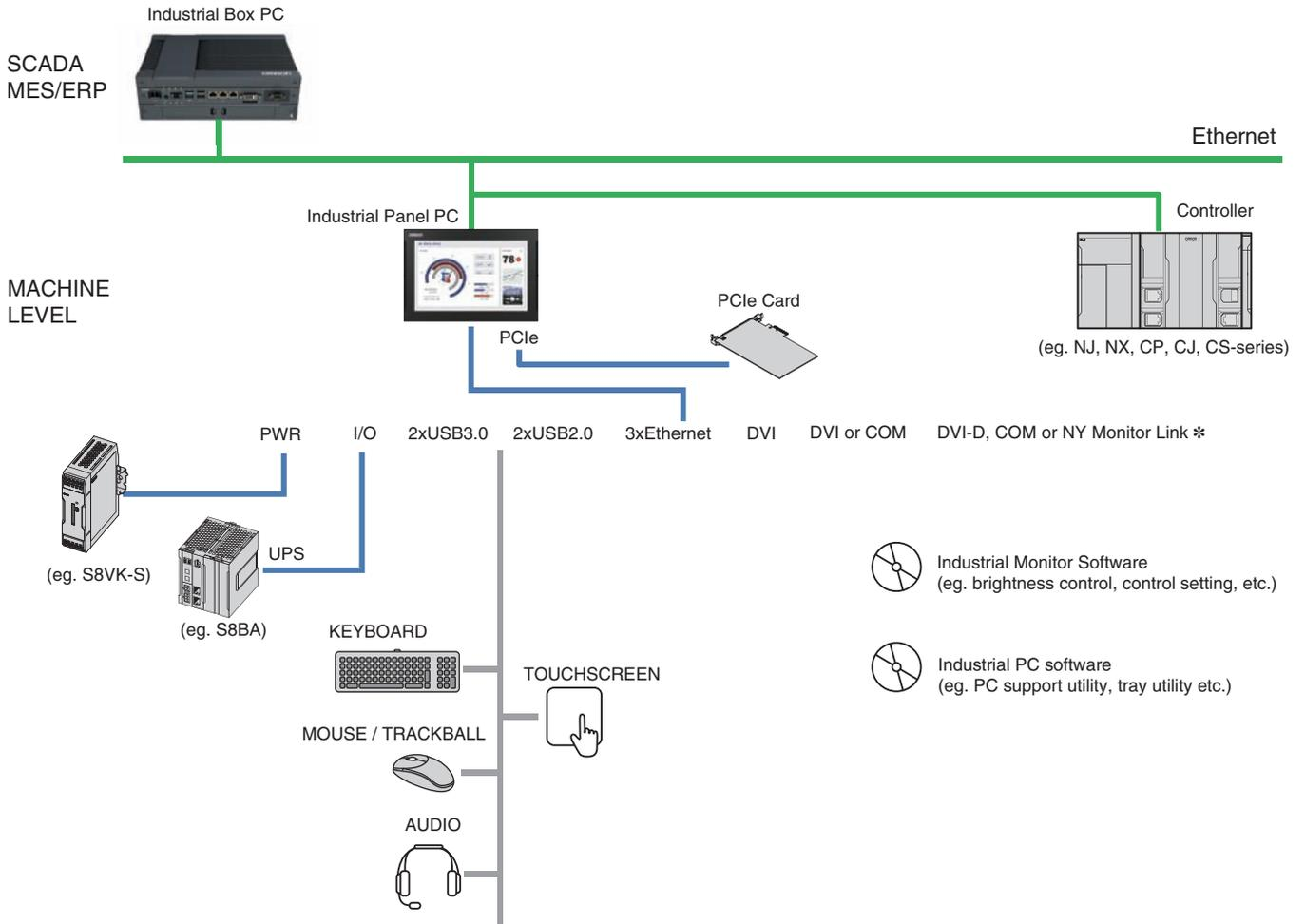
\* NY Monitor Link option: Connect monitor up to 100 m via standard Ethernet cable.
