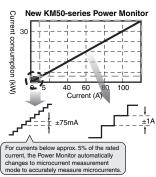
You can measure microcurrents of  $\pm 75$  mA with a CT with a rated current of 100 A. (Reference Value)
