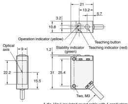
4-dia. Vinyl-insulated round cable with 4 conductors (Conductor cross section: 0.2 mm² (AWG.24), Insulator diameter: 1.1 mm), Standard length: 2 m
