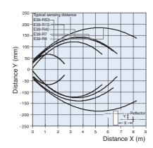
Retro-reflective Models (radial) E3F2-R2R□41-□ (polarizing) and reflectors
