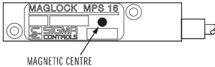
The magnetic centre of a Maglock switch or actuator is denoted by a symbol on the operating face as indicated in the diagram.
