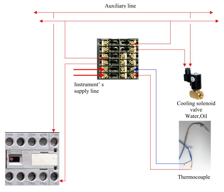
Contactor for heating power
