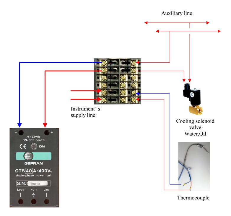
Heating control scheme with solid state relay and fan pilotage for cooling zone
