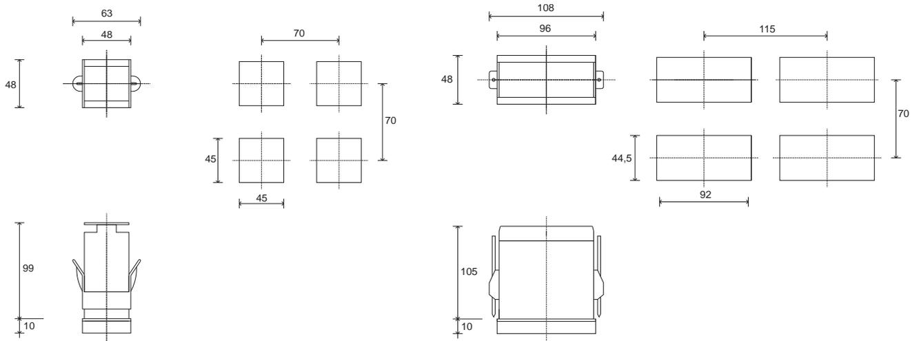
Face avant: 48x48mm - 96x48mm (1/16DIN - 1/8DIN). Profondeur 99mm - 105mm
