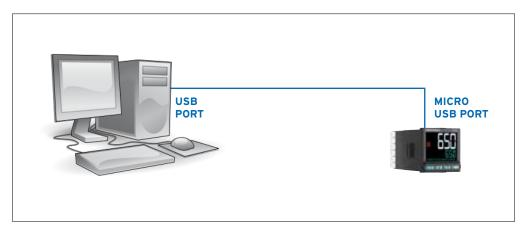
This connection requires a MicroUSB/USB cable conversion for connection between the PC on which GF\_eXpress is installed and the device to be configured
