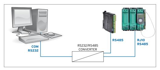
This connection requires a RS232/RS485 converter and connection cables for connection between the PC on which GF\_eXpress is installed and the device to be configured.
