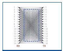
SCAN MODE 3-4: low speed / high resolution Minimum object detection Flat = 0.2 (thickness) x 75 (width) mm Cylindrical objects = Ø 6 mm
