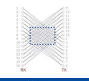
SCAN MODE 2: high speed / mid resol. central area Minimum object detection Flat = 0.4 (thickness) x 90 (width) mm Cylindrical objects = Ø 6 mm
