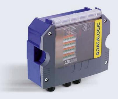
CBX800 is an industrial gateway allowing connection of devices equipped with a standard RS232 communication interface to the most common fieldbus systems, by means of a complete range of optional modules, and to ID-NET™ high speed communication network. CBX800 allows, with the same model, flexible interfacing of several devices (e.g. Datalogic Automation's 6K and 8K series, Hand Held Readers) to different networks.
