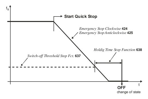
If frequency/speed reaches the value zero during the switch-off time, the drive continues to be supplied with current until the switch-off time has elapsed. This ensures that the drive is at a standstill when the state changes.
