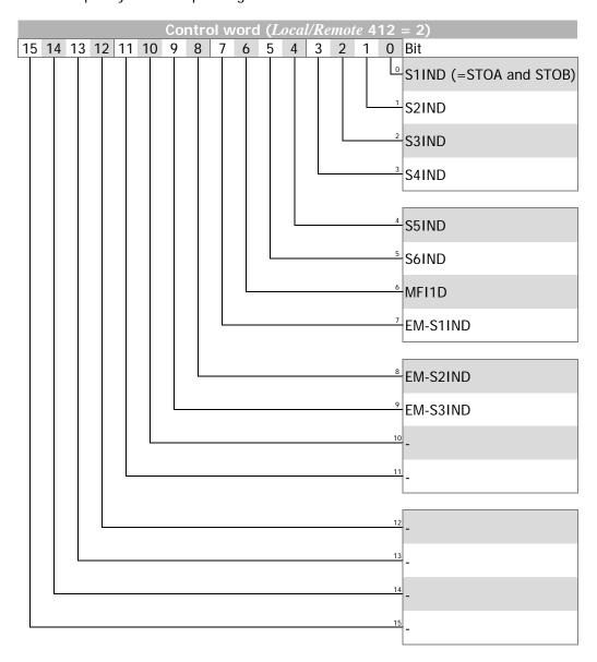
The digital inputs set via the control word can be monitored using parameter *Digital inputs* **250**. Digital input S1IND will only be displayed if controller release is switched on at STOA and STOB **and** the control word (Bit 0) was set. If the data set switching function is used, please ensure that Parameter *Local/Remote* **412** is set to "2 – Control via remote contacts" is set in all data sets used.
