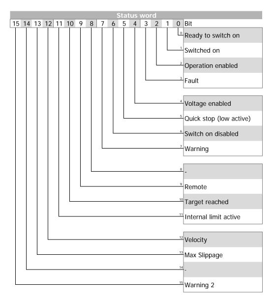
The Profile Velocity Mode is used to set the reference speed in user units [u/s]. The reference speed PZD5/6<sup>r)</sup> *Profile Velocity* is taken over in mode "operation enabled" immediately (0xnn37). The acceleration and deceleration ramp are specified by PZD7/8<sup>r)</sup> *Profile acceleration* and PZD9/ $10^{r)}$  *Profile deceleration*.
