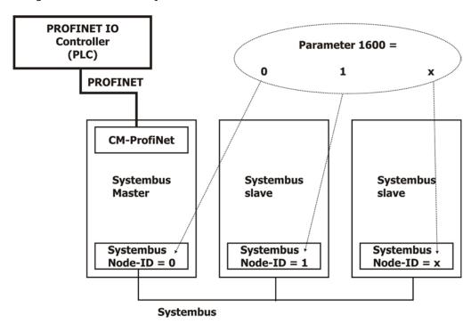
In order to access the parameters of the individual frequency inverters through System Bus, Parameter **1600** is set to the ID of the relevant Systembus node.
