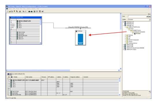
The two possible objects PKW and PZD are available in the **BV Drive** menu. The required object can be assigned to the frequency inverter (drag & drop).
