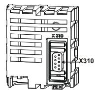
The bus socket **X310** (9-pole Sub-D) is connected according to the Profibus DP standard EN50170.
