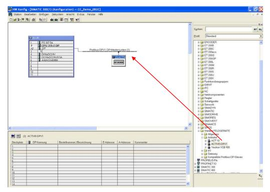
The six possible objects PPO1 to PPO4 and PKW, PZD are visible under the menu item **ACTIVE-DPV1**. The required object is now assigned to the inverter by Drag & Drop.
