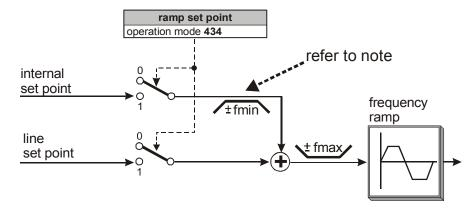
The internal set point value from the reference frequency channel and the line set point value can be fed to the ramp individually or as an added variable. The setting is carried out via the data set change-over capable parameter *Ramp set point* **434**.
