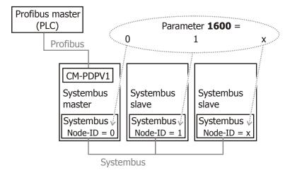
To obtain access to parameters of inverters via the Systembus, parameter **1600** is written to the desired Systembus node ID.
