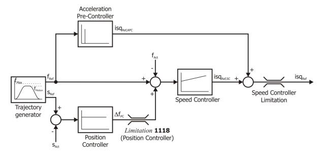
In order to avoid oscillations of the drive while it is at standstill, amplification is reduced to 50 % of the parameterized value for small position deviations.
