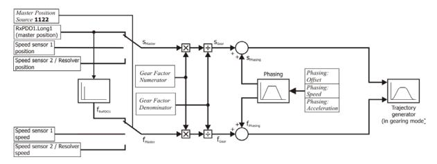
The master position and speed are multiplied by the *gear factor*. When phasing is started, the phasing profile is added to the master speed until the phasing offset is reached.
