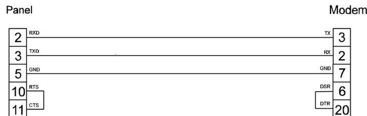
figure 1. Cable diagram
