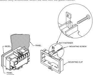
While holding the unit in place, push the panel latch over the rear of the unit so that the tabs of the panel latch engage in the slots on the case. The panel latch should be engaged in the farthest forward slot possible. To achieve a proper seal, tighten the latch screws evenly until the unit is snug in the panel (Torque to approx. 28 to 36 in-oz [0.202 to 0.26 N-m]). Do not over-tighten the screws.
