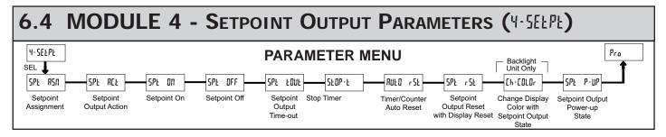
The Setpoint Output Parameters are only active when the optional relay module is installed in the meter. Some parameters will not appear depending on the Setpoint Assignment and Setpoint Output Action selected.
