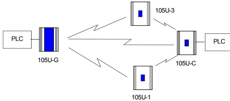
105G modules can transmit to 105G modules as well as other 105G modules. There can be multiple 105G and 105C modules in a network - as well as 105U I/O. Because the 105U protocol is peer-to-peer, there are few constraints on communications between multiple 105U modules.
