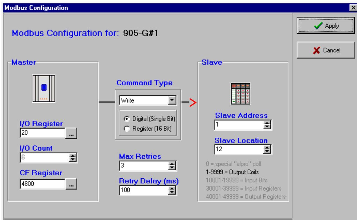
To enter a Modbus command, select “New Serial Mapping”. The following example is a digital write command which writes 105G I/O registers 20 – 25 (6 registers) to Modbus outputs 00012 – 00017, at Modbus Slave address 1.
