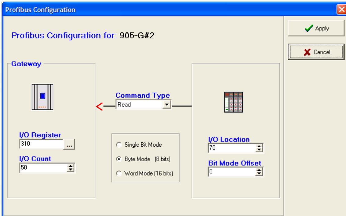
The third link is a “byte read” link - a block of 50 bytes are read from Profibus byte 70 – 119, and stored in I/O registers 310 – 359. The 8-bit values of each byte are stored in the most significant 8-bits of the I/O register.
