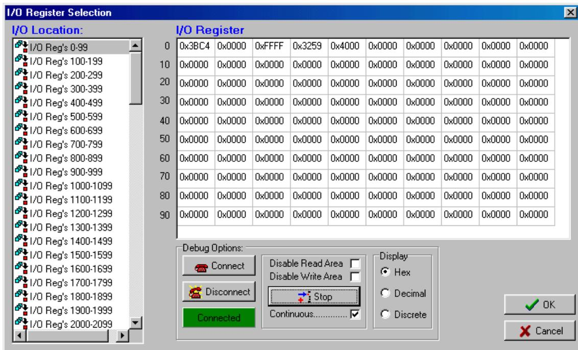
To write to a register double click with mouse on the register and a pop up box will appear as shown below. Enter value and press 'OK'.
