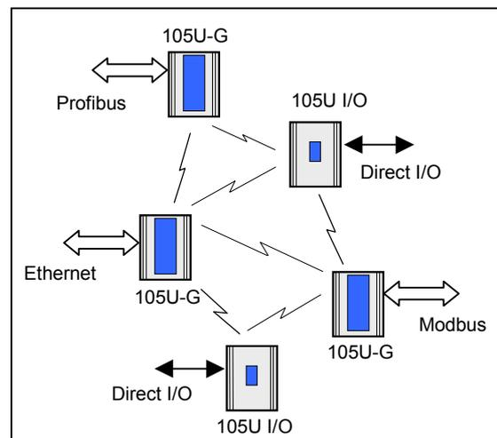
The 105U-G has eight on-board discrete I/O. Each I/O point can be configured individually as a contact input signal, or a discrete output signal. Input signals can be sent via its data-bus connection to a host device (PLC, DCS etc) or be transmitted by radio to other 105U units. The output signals can be driven by a host device, or linked to inputs on remote 105U units.
