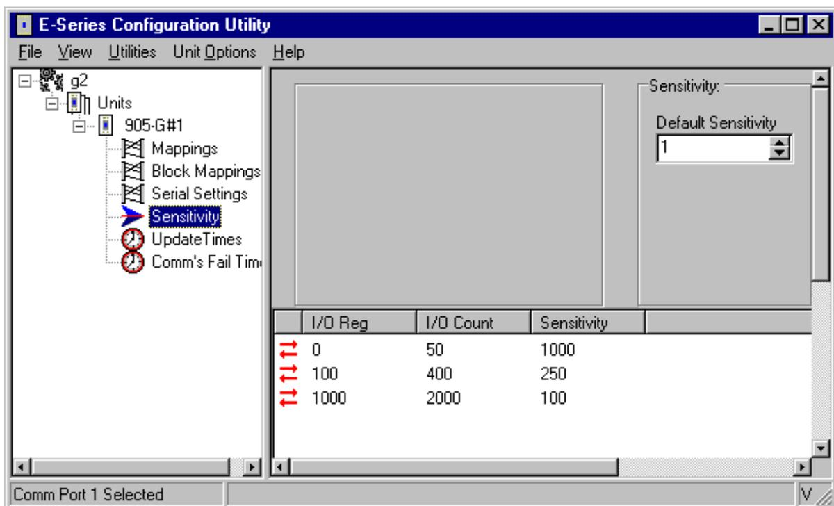
value to trigger the message. Sensitivities are configured for blocks of I/O registers - that is, each I/O register does not have a unique sensitivity. You can configure up to 50 sensitivity values - that is, there can be 50 blocks of registers with different sensitivities.
