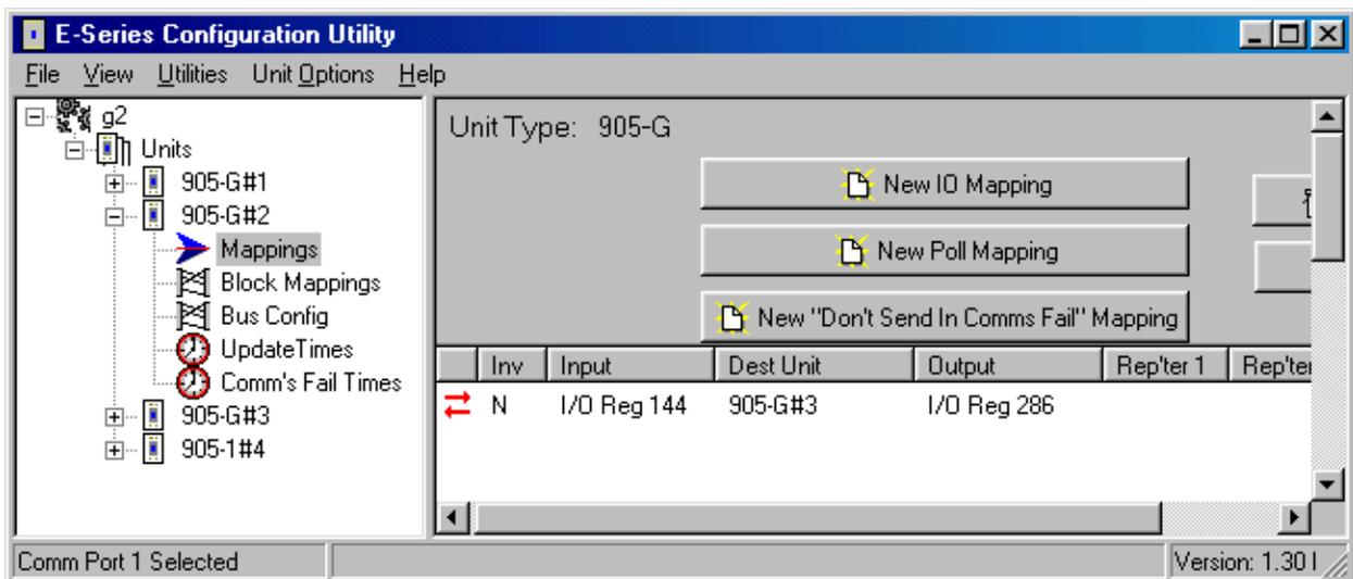
Whenever I/O Reg 144 changed by the sensitivity amount, 105G#2 would send a message to 105G#3 to write the value in I/O Reg 286. The problem arises if there are a lot of these mappings. Each radio message only relates to one register-register link. If you want to map 1000 registers from one 105G to another, then this could generate a lot of radio messages.
