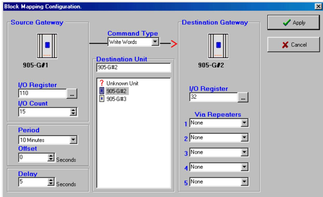
Select the “Command Type” from the pop-down window in the centre of the display. The red arrow will confirm the direction of the block transfer. Now select the destination module - only the 105G modules already configured will be shown. If you need to use repeaters in the radio link, enter the repeater addresses, starting with the repeater closest to the source module.
