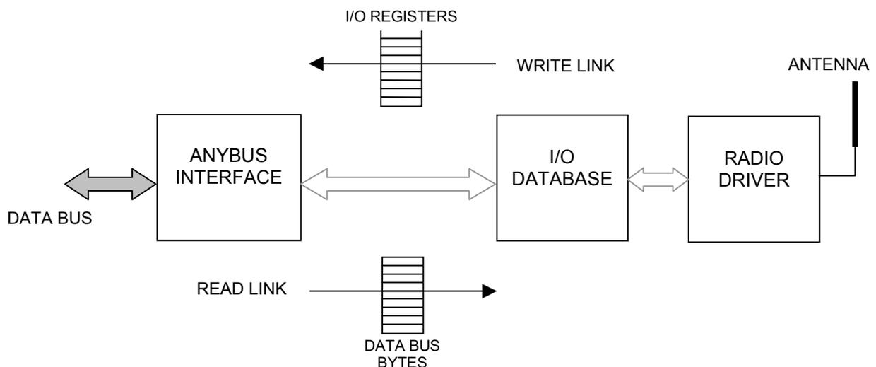
A Read Link reads values from Anybus “output” bytes and stores the values in I/O registers. If the host device wants to send a value to the 105G, it will write to the Profibus output bytes - the 105G will then transfer these values to the I/O data base using a Read Link.
