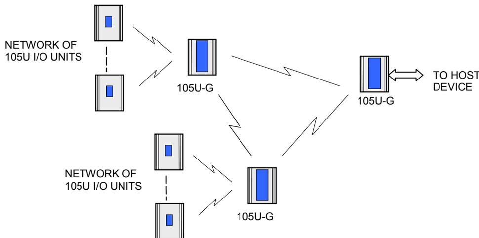
This type of network reduces the amount of radio traffic and is suitable for systems with a large number of I/O modules. The system is divided into local sub-networks, each with a 105G unit. The 105U modules transmit their I/O values to the 105G. The 105G then transfers these values to the “central” 105G using a block transfer which is very efficient compared to a lot of individual I/O transmissions.
