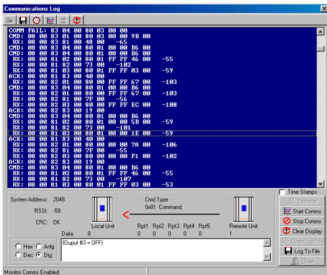
The display will show radio messages transmitted and received. Messages starting with RX are received messages, CMD are transmitted messages and ACK are acknowledgement messages. At the end of each message is the RSSI (radio signal strength) in dBm.
