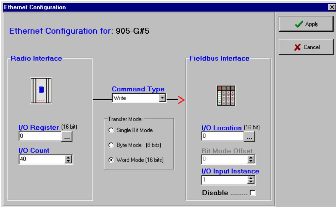
In this example, 40 I/O Registers (80 bytes) are transferred to I/O Input Instance 1 (i.e. Ethernet connection 1). As per the table below, this data would then be available via Ethernet/IP in class 04h, Instance Attribute 64h *or* in class A0h, Instance Attribute 1. If the *Disable* option is checked, the I/O transfer will not be made available to Ethernet/IP. The table below shows the possible IO Instances and their corresponding Ethernet/IP locations.
