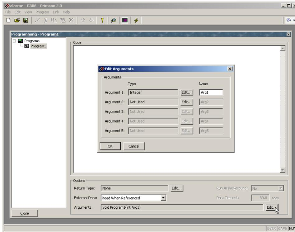
Now the OnHelp field is ready to accept the following code. This tells the viewer to run **Program1** with the information provided in **Data** when the Help button is pressed.
