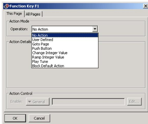
You will note that this dialog box has two tabbed pages. The first page is used to define what will happen when the key in question is pressed when the current page is selected. The second page is used to define what will happen if the key is pressed when any page is selected. The first type of action is called a *local* action, while the second type is called a *global* action. The color used to display the key will change according to which actions are defined...
