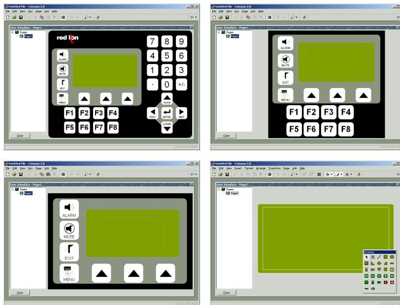
As you can see, at each level, fewer keys are shown, and more of the window is allocated to the display itself. The zoom level can be controlled from the View menu, by using the magnifying glass icon, or by pressing the **Alt** key together with the digits **1** through **4**.
