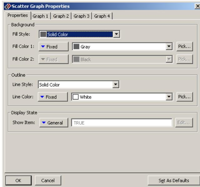
Each graph is composed of the same proprietary set of properties. Data sources and scaling are defined directly on the graph tab. The format and style are accessible via the Edit button.
