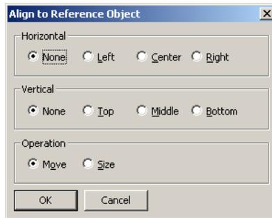
The Horizontal and Vertical settings can be used to indicate what type of alignment is to be performed, while the Operation setting indicates whether the primitives should be resized or moved to achieve the desired result.
