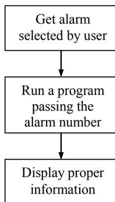
The first step is achieved using the system variable **Data**. This system variable is only available for the OnHelp field and contains information on the alarm selected. **Data** is a Long (Double word) and contains the following information:
