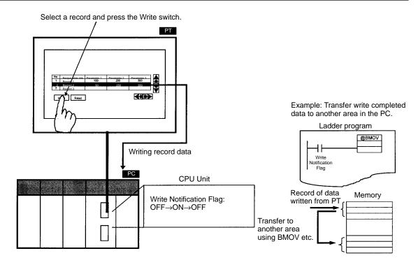
**Reference:** Recipe tables and recipe elements are stored in flash memory within the PT and memory (recipe data memory) that is backed up by a battery. The way that the data is stored is explained below and illustrated in the diagram following.
