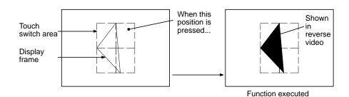
There are four standard touch-switch guide characters: fixed display character strings, ON/OFF switching character strings, numeral displays, and character string displays. When fixed display character strings or ON/OFF switching character strings are used, several lines of guide characters can be displayed.
