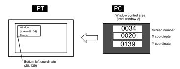
When the window display status changes, the change is notified to the window control area as shown below (Window's Opening/Closing status is notified to the PT status notify area as well).
