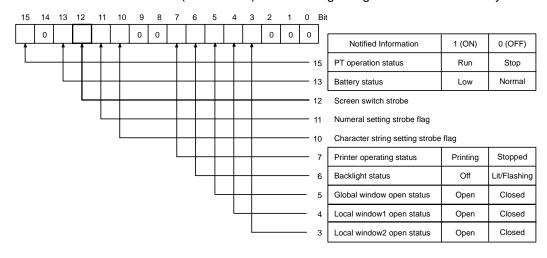
To check the operating status of the printer, operate the PT status notify area in the manner shown below.
