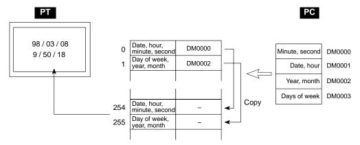
To copy a memory table, either use the PT status control area or the touch switch copy setting function. Here, the procedure for copying a memory table using the PT status control area is described. For the procedure for using the touch switch copy setting function, refer to Changing Numeric Values/Character Strings by Pressing a Touch Switch Which Has the Copy Setting Function (page 315).
