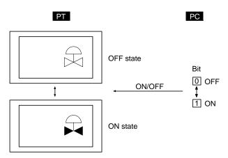
Create figures depicting the valve when open (A in the figure below) and the valve when closed (B in the figure below), either by using library data (fixed display graphic) or image data (comprised of dots).
