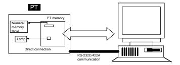
In the memory link method, the only difference is that the PT finds its communication target inside instead of outside. In the memory link method, therefore, change of the target is all that is needed to be capable of using the exact screen data that is acquired by the direct connection. (With the NT31/NT31C and NT631/NT631C, the Support Tool must be used to convert the data to screen data for the memory link.)
