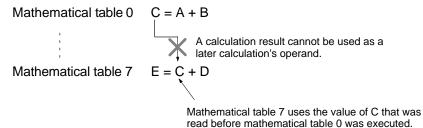
The mathematical function's processing cycle does not match the PC's cycle time, so results from two calculations may not be from the same processing cycle.
