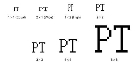
With ISO 8859-1 font type, the character strings of  $2 \times 2$  or larger scale are automatically displayed in 32 dot high-definition font. However, the marks inserted into a string are always displayed in  $16 \times 16$  dot font.
