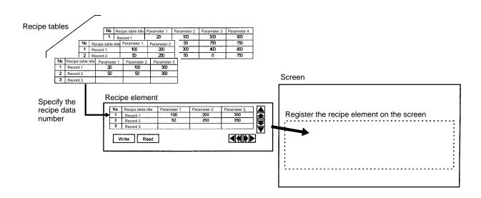
Sending Recipe Tables and Recipe Elements Using the Support Tool Send recipe tables (i.e., entire sets of recipe data) and recipe elements created as shown above from the Support Tool to the PT in application units (i.e., send all screen data in a single operation).
