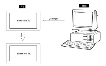
Use PT memory write command (sent from host to PT) for this case since it is necessary to write new screen number to the first word in PT control area.
