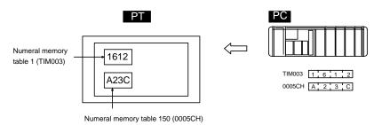
Allocate numeral memory tables to any desired words in the PC. If the contents of the allocated words are changed while the numeral memory table data is being displayed on the screen as numeric values or lamps, the corresponding display on the screen will also change automatically. This function allows the contents of allocated words to be monitored easily.
