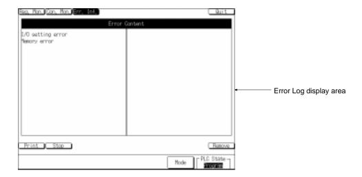
With the NT631/NT631C, 30 error records (15 records  $\times$  2 columns) can be displayed in one screen. The highest priority error must be cleared in order to display the thirty-first error record.
