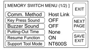
Each time the "Key Press Sound" touch switch is pressed, the setting option "ON" alternates with "OFF".
