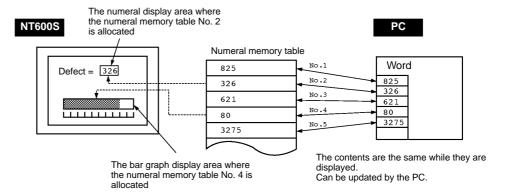
During the operation, the display contents are automatically updated so that the contents of the numeral memory table being displayed are the same as that of the PC word.
