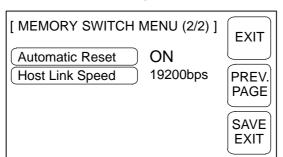
Each time the "Host Link Speed" touch switch is pressed, the setting option "9600 bps" alternates with "19200 bps".
