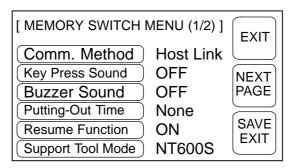
Each time the "Comm. Method" touch switch is pressed, the setting option changes to the next item in the sequence "Host Link", "NT Link", "NT Link 1:N", "RS-232C".
