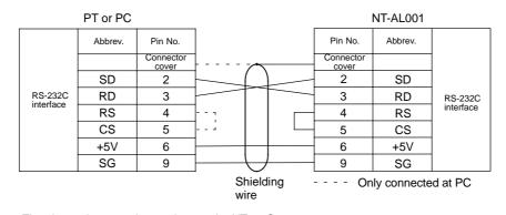
The pin numbers are the numbers at the NT600S. For the pin numbers at the PC, refer to the manual for the PC used.
