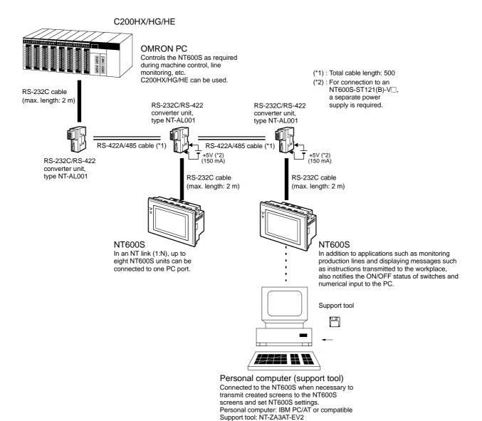
Reference When connecting the C200HX/HG/HE and an RS-232C/RS-422 converter unit, use a converter unit whose lot number is 15Y5 or later. Converter units of lot numbers previous to 15Y5 cannot be connected.
