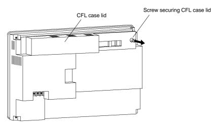
2. Disconnect the backlight connector from the NT600S.
