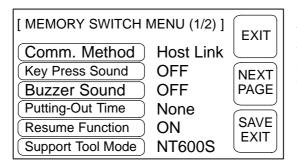
Each time the "Putting-Out Time" touch switch is pressed, the setting option will switch among "10 min", "1 hour", and "None".
