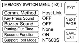
Each time the "Support Tool Mode" touch switch is pressed, the setting option changes from "NT600S" to "NT600M" or from "NT600M" to "NT600S".
