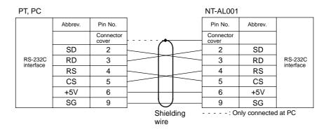
The pin numbers are the numbers at the NT600S. For the pin numbers at the PC, refer to the manual for the PC used.
