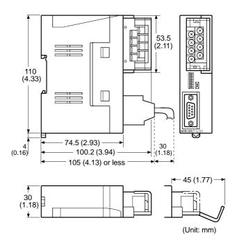
With RS-422A terminal block cover closed: 30 (W) x 114 (H) x 100.2 (D) mm With RS-422A terminal block cover open: 30 (W) x 114 (H) x 119.5 (D) mm
