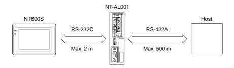
Reference When connecting a C200HX/HG/HE and an RS-232C/RS-422 converter unit, use a converter unit whose lot number is 15Y5 or later. Converter units of lot numbers previous to 15Y5 cannot be connected.
