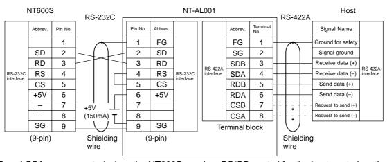
(\*) CSB and CSA are connected when the NT600S requires RS/CS control for the host control method.
