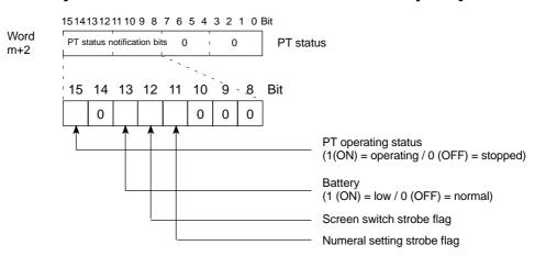
The NT600S statuses that the PC can determine are listed below.
