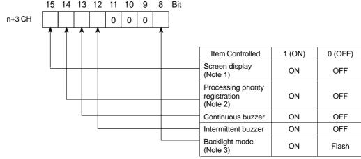
Note 1: When "ON" is set for screen display, the backlight/EL display is on; when "OFF" is set for screen display, the backlight is off.
