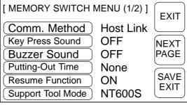
Repeatedly pressing the "Buzzer Sound" touch switch cycles through the setting options "ON", "ERR ON", and "OFF".
