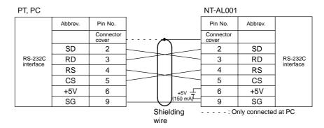
The pin numbers are the numbers at the NT600S. For the pin numbers at the PC, refer to the manual for the PC used.
