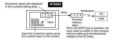
If there is more than one numeral setting area, the one in which the numerical value is to be input can be selected by using a touch switch (numeric key).
