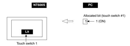
The status of the control bit reflects the touch switch status, as follows:
