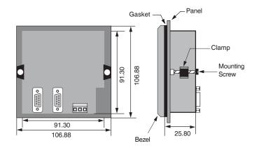
NT3S-ST121B-E, NT3S-ST123B-E, NT3S-ST124B-E, NT3S-ST126B-E Panel cutout: 132.00 mm x 69.00 mm All dimensions are in mm.
