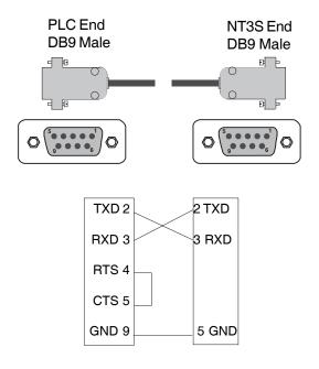
Pin Configuration for communication cable between Omron plc RS232 port and NT2S-SF121/SF125:
