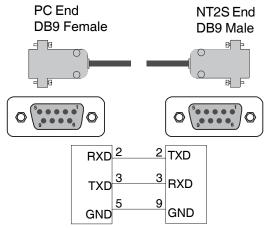
Pin Configuration for communication cable between Omron plc RS232 port and NT3S:
