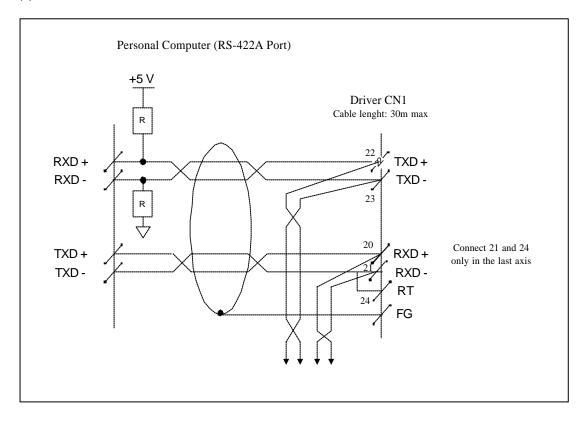
Connect the shield to the frame ground inside the Servodriver through the connector case. When executing communications for multiple axles, the Driver frame grounds must be connected to the same point.
