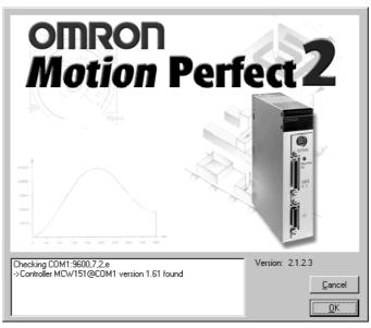
The status of the connection to the controller is displayed on the screen. The statements indicate at which COM port Motion Perfect is currently checking for a Motion Controller and which settings are used. The screen will confirm if Motion Perfect has found a controller or will indicate that no controller is found.
