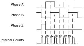
The Z-phase signal has the following specification:
