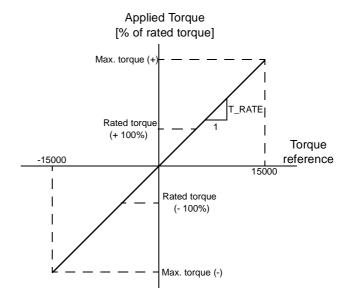
The torque characteristics are Servomotor dependent. The actual applied torque of the Servomotor as percentage of the rated torque can be determined by using the T\_RATE axis parameter.
