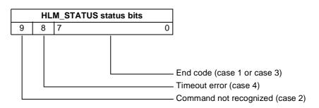
If no error did occur the HLM\_STATUS will have value 0. In case of a nonzero value, any appropriate action such as a re-try or emergency stop needs to be programmed in the user BASIC program.
