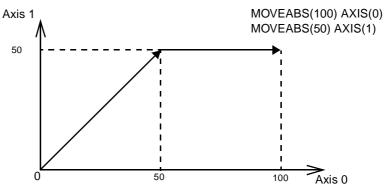
At start, both the axis 0 and axis 1 will move to a coordinate of 50 over the same duration of time. At this point, axis 1 will stop and the axis 0 will continue to move to a coordinate of 100.
