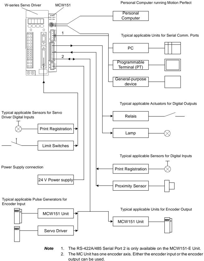
The equipment and models which can be used in the system configuration are shown in the following table.
