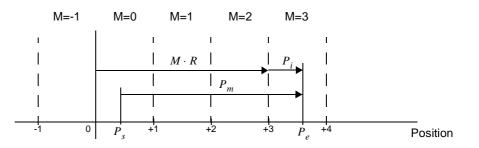
At start-up the internal measured position of the MC Unit will be determined by using the following formula.
