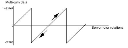
With any other setting than 65535, the Servomotor multi-turn data will be as follows:
