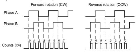
The signals A, B and Z appear physically as A+ and A-, B+ and B- and Z+ and Z-. These appear as differential signals on twisted-pair wire inputs, ensuring that common modes are rejected and that the noise level is kept to a minimum.
