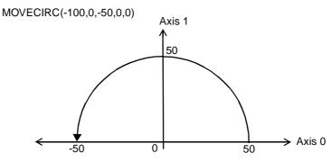
The centre point and desired end point of the trajectory relative to the start point and the direction of movement are specified. The MOVECIRC command computes the radius and the angle of rotation. Like the linearly interpolated MOVE command, the ACCEL, DECEL and SPEED variables associated with the base axis determine the speed profile along the circular move.
