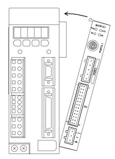
When removing the MC Unit, press down the top of the MC Unit case and remove the upper extension from the Driver.
