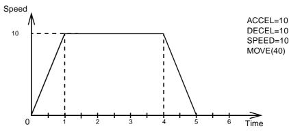
The following two speed profiles show the same movement with an acceleration time respectively a deceleration time of 2 seconds.
