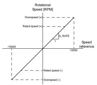
The speed characteristics are Servomotor dependent. The S\_RATE axis parameter specifies the speed reference rate of the attached motor. This rate is defined as the amount of Rotational speed (in RPM) per unit of speed reference.
