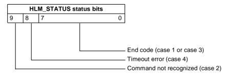
If no error did occur the HLM\_STATUS will have value 0. In case of a nonzero value, any appropriate action such as a re-try or emergency stop needs to be programmed in the user BASIC program.
