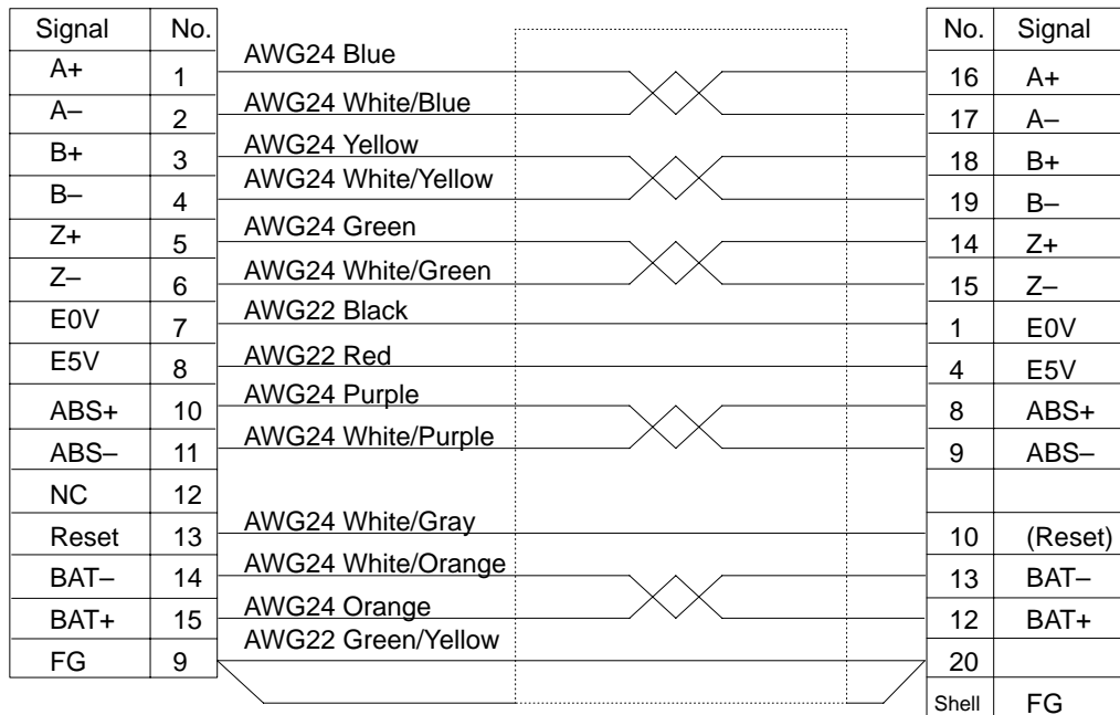
Cable: AWG22 × 3C + AWG24 × 6P
