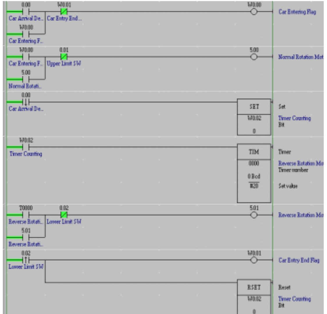
By the procedures so far, the ladder is running and the condition set in IO Condition Configuration is monitored by the virtual PLC. After this, pseudo input of car arrival and gate passing is executed and debug of a ladder program is executed.
