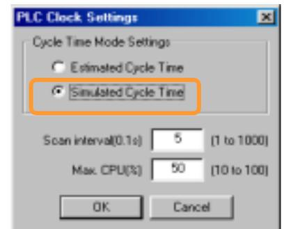
The default cycle time information in CX-Simulator is set to "Simulated Cycle Time" which is the time for running a program on an active PC. To check the estimated cycle time when running a program on an actual PLC, change "Cycle Time Mode Settings" from "Simulated Cycle Time" to "Estimated Cycle Time" in the PLC Clock Settings of CX-Simulator.
