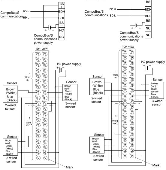
**Note** 1. The V terminals are all connected internally, as are the G terminals.
