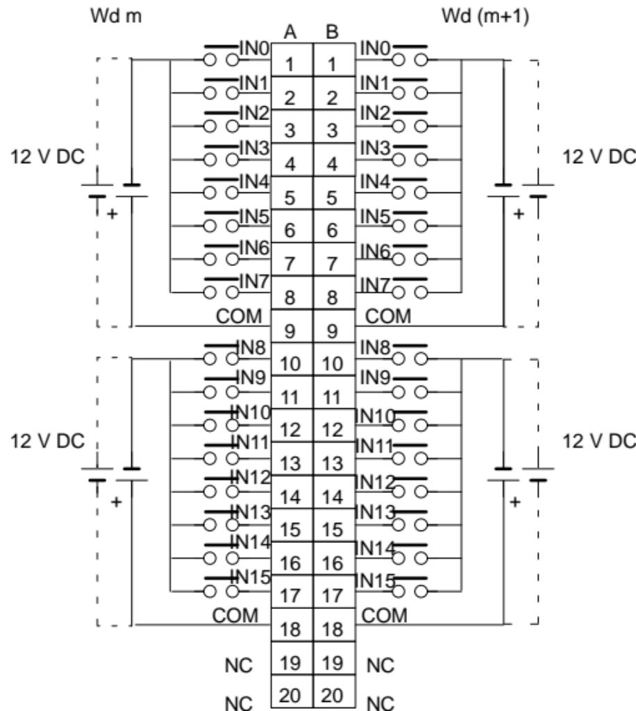
The polarity of the input power supply can be either plus or minus. The polarity of all the commons, however, must match.
