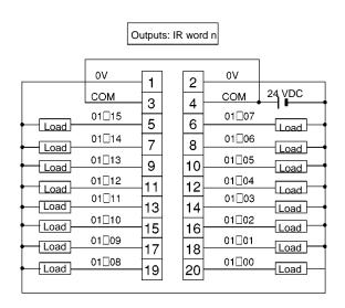
**Note** Wire COM terminals (3 and 4) and 0-V terminals (1 and 2) even though they are connected internally.
