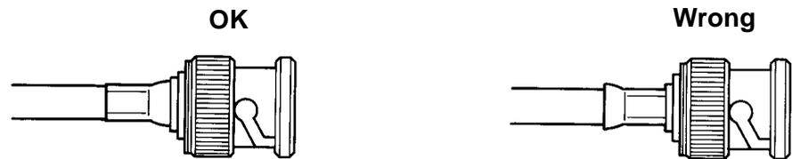
Check that the contact tip is in the same position as the open mouth of the connector.
