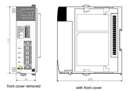
The CQM1-ARM21 is an AS-Interface master unit for OMRON's CQM1 range of programmable controllers. It can be mounted to any CPU type of the CQM1 series, within the restrictions for the number of I/O channels available in that CPU.
