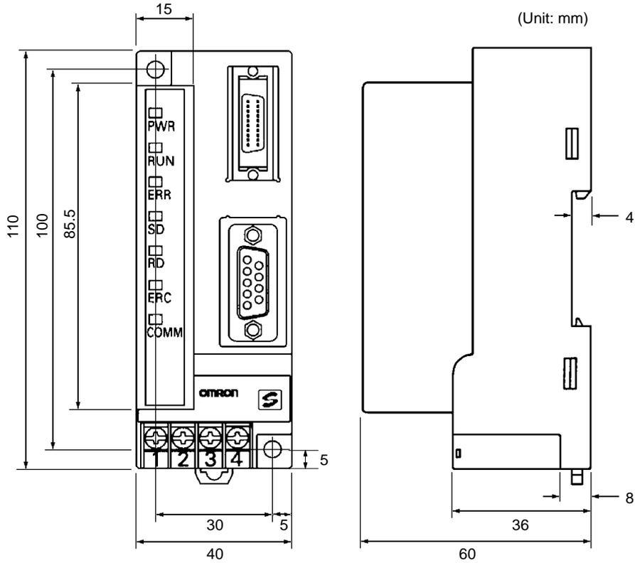
When mounting a Peripheral Device, be sure to allow sufficient space as shown in the following diagram.
