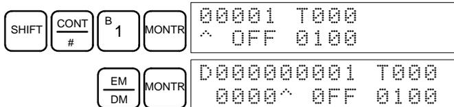
If 4 or more bits and words are being monitored, the bits and words that do not appear on the display can be displayed by pressing the MONTR Key. If the MONTR Key is pressed alone, the display will shift to the right.
