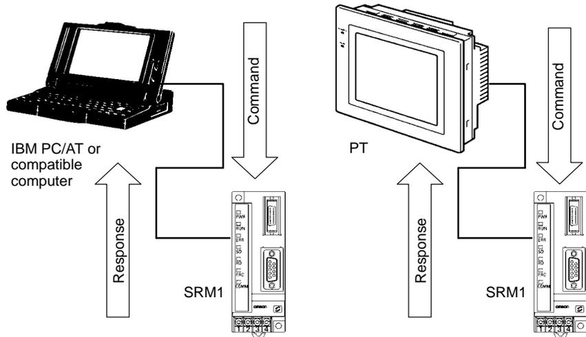
**One-to-one Host Link Cables** The cables differ depending on whether the peripheral port or RS-232C port is used.
