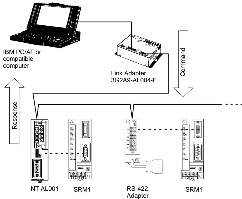
**One-to-N Host Link Cables** Up to 32 SRM1s can be connected to the computer via the peripheral port or RS-232C port.
