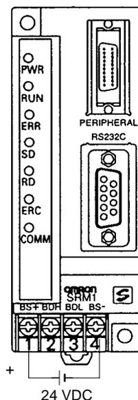
**Note** Be sure to ground the ground terminal of the power supply.
