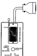
CPM1-EMU01-V1 | Expansion Memory Unit     | Uploads the ladder program and DM 6144 to DM 6655 from the PC to the EEPROM and downloads the ladder program and DM 6144 to DM 6655 from the EEPROM to the PC. |                   |
