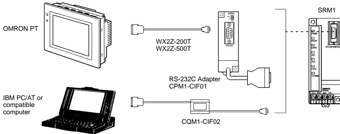
**Note** Set the RS-232C Adapter mode setting switch to "HOST."
