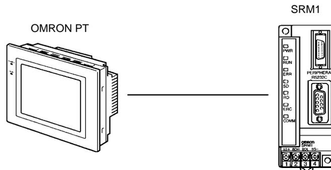
The 1:N NT Link is possible only with the SRM1-C02-V2 PCs, which have an RS-232C port.
