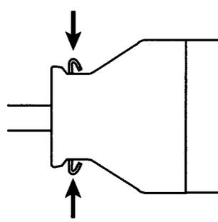
**Note** Do not attempt to remove the connector by pulling the cable.
