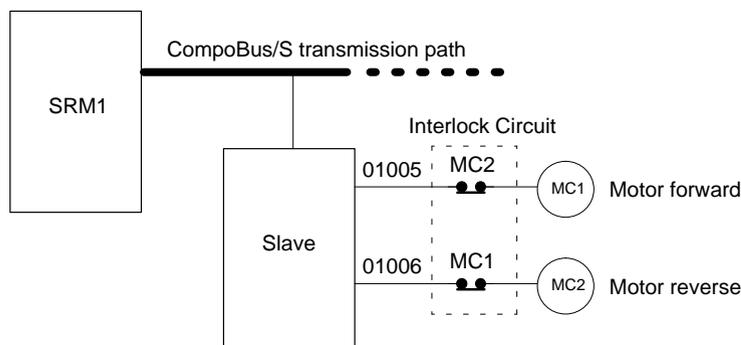
In the interlock circuit above, MC1 and MC2 cannot be ON at the same time even if SRM1 outputs 01005 and 01006 are both ON at the same time (an incorrect operation).
