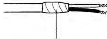
Secure the cable sheathing with electrical tape or heat-shrink tubing.
