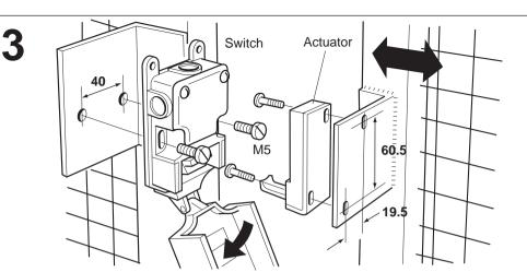
Hinge down the cover to gain access to the mounting holes. Mount the switch on the stationary section of the guard using 2 x M5 fixings. Use mounting brackets if necessary.
