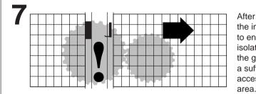
After installation check all of the interlocked guard doors to ensure that the machine is isolated and stopped before the guard has been opened a sufficient distance to allow access to the hazardous
