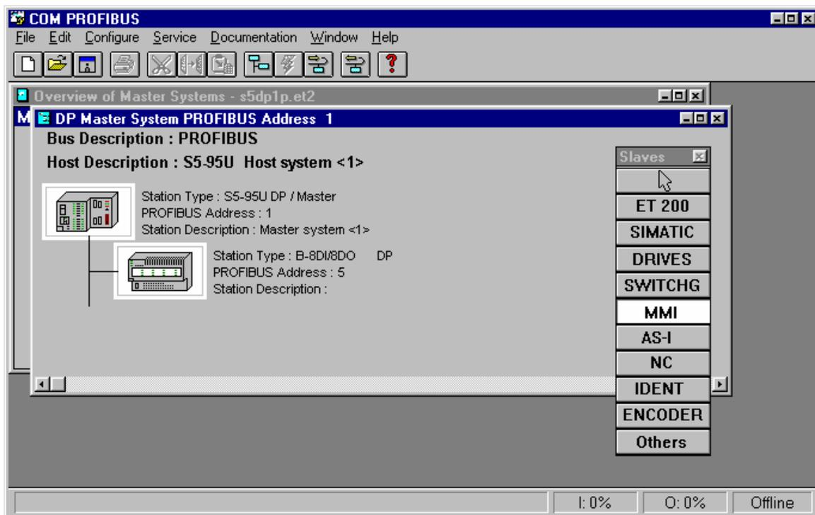
Figure 4 - COM Profibus Network Configuration Editor
